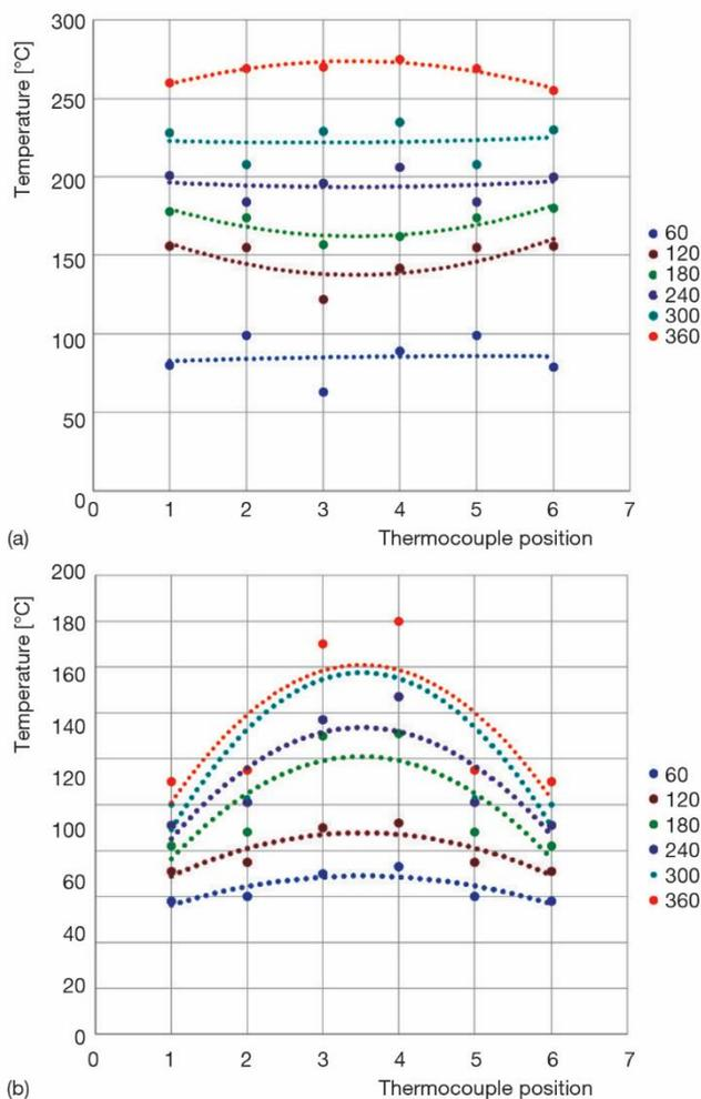
**Figure 6. Temperature profile over the plate surface (case with  $\delta = 20$  mm thickness); effect of the burner type; (a) heating by a microflare burner and (b) heated by the conventional gas burner**
