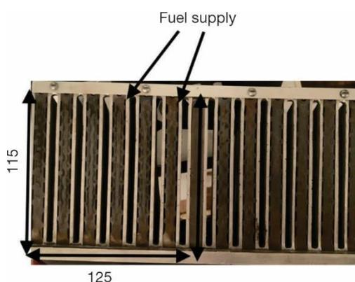
**Figure 2. View of the burner**
