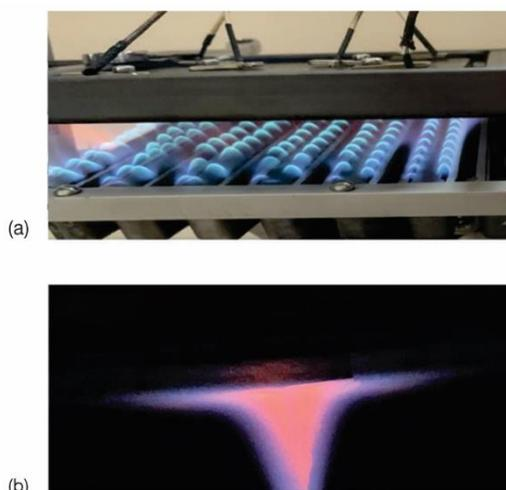
**Figure 8. Photos of the burner used; (a) a microflare burner and (b) a conventional gas burner**
