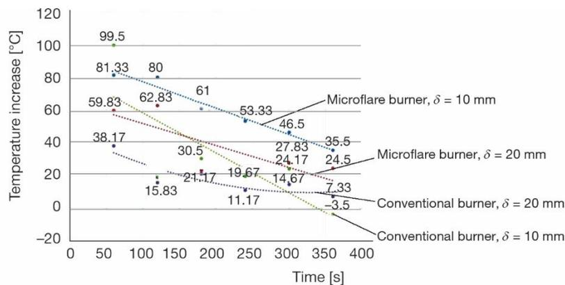
**Figure 7. Average plate temperature evolution in time; (a) heating by a microflame burner and (b) heated by a conventional gas burner**
