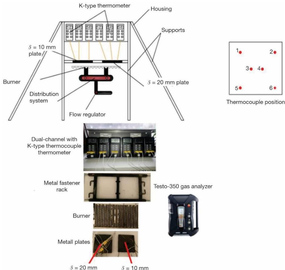
**Figure 1. Experimental installation**
