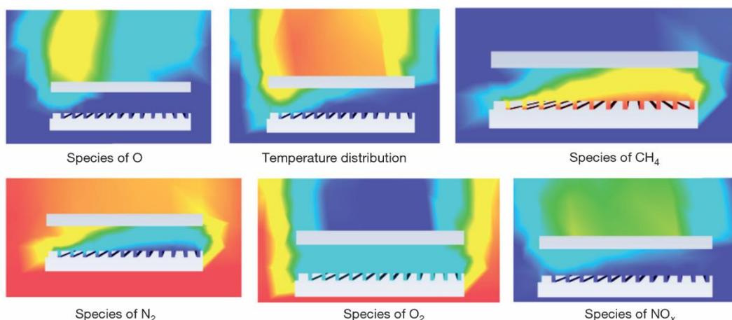
Figure 11. Distribution of temperature and species for microflame burner
