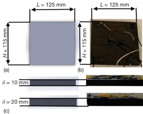
**Figure 3.** Plates used in the experiments (simulations and physical); geometrical (a), physical (b) models, and views correspondingly (c)
