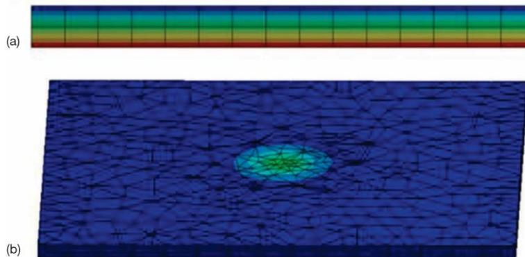
Figure 10. Temperature field of the heated metallic plates; (a) microflame burner and (b) conventional burner
