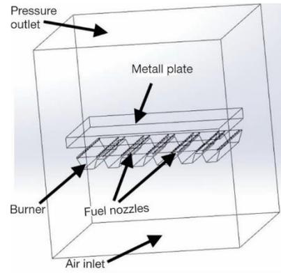
**Figure 4.** Schematic presentation of the simulated combustion chamber
