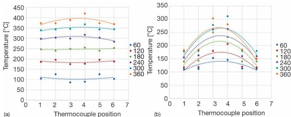
**Figure 5.** Temperature profile over the plate surface (case with  $\delta = 10$  mm thickness); effect of the burner type; (a) heating by the microflare burner and (b) heated by the conventional gas burner
