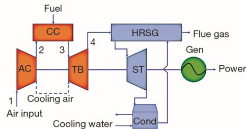
Figure 2. Schematic of the NGCC power plant system
