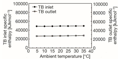
Figure 7. Variations of specific enthalpies of flue gas at TB inlet and outlet
