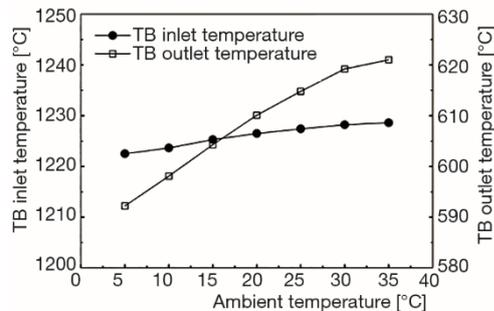
Figure 4. Variations of TB inlet and outlet temperature against ambient temperature
