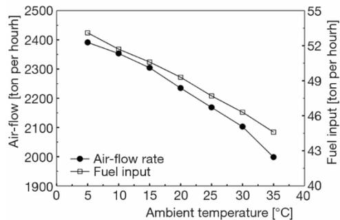
Figure 8. Variations of air-flow rate and fuel input rate
