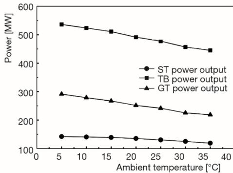
Figure 5. Variations of power output of ST, TB, and GT
