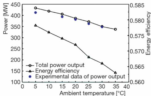
Figure 3. Variations of NGCC power output and energy efficiency
