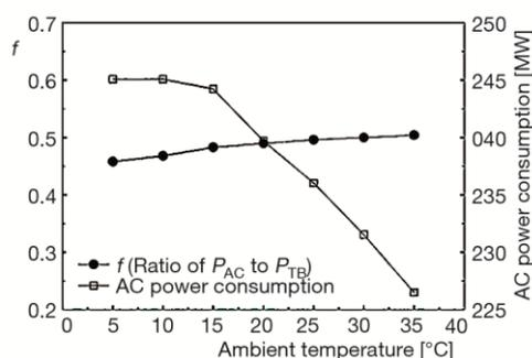
**Figure 9. Variations of  $f$  and AC power consumption**
