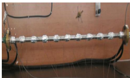
Figure 2. Attachment of thermocouples to the test pipe
