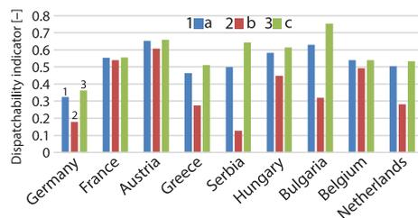
**Figure 6. Dispatchability indicator for three portfolio's technology structures; (a) base; (b) HCfPP and LfPP substituted with WG, and (c) HCfPP and LfPP substituted with NPP**
