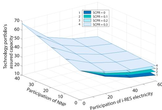
**Figure 2. Technology portfolio's assured capacity (at the power system's level) as function of  $\beta$  and  $\lambda$  indicators**
