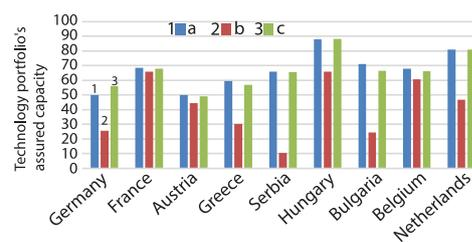
**Figure 7. Technology portfolio's assured capacity for three portfolio's technology structures; (a) base, (b) HCfPP and LfPP substituted with WG, and (c) HCfPP and LfPP substituted with NPP**
