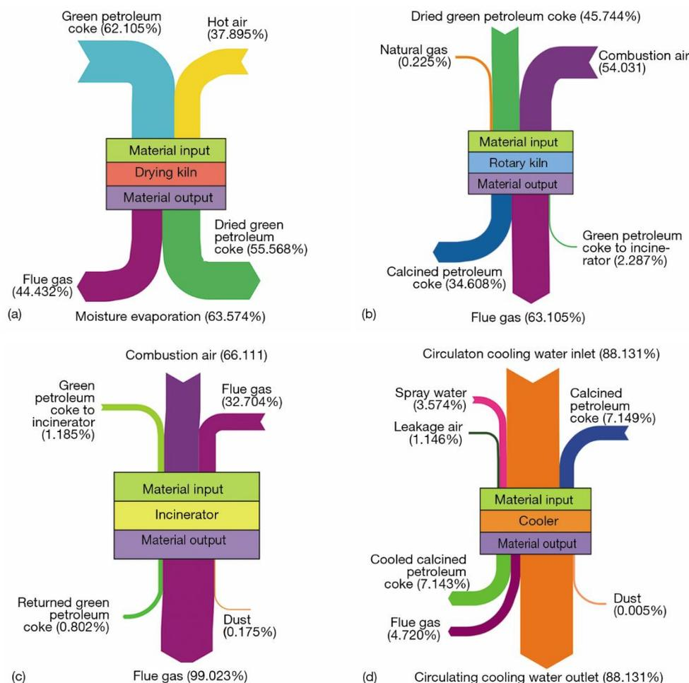
**Figure 2. Sankey diagram of material flow in the four different equipment; (a) Sankey diagram of the material flow in the drying kiln, (b) Sankey diagram of the material flow in the rotary kiln, (c) Sankey diagram of the material flow in the incinerator, and (d) Sankey diagram of the material flow in the cooler**
