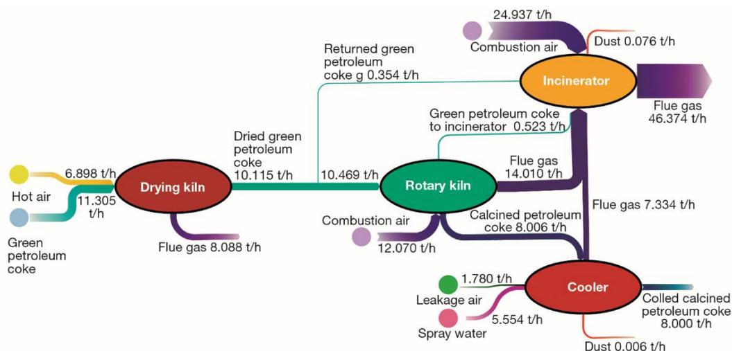
Figure 4. Sankey diagram of the material flow with the suggested improvements
