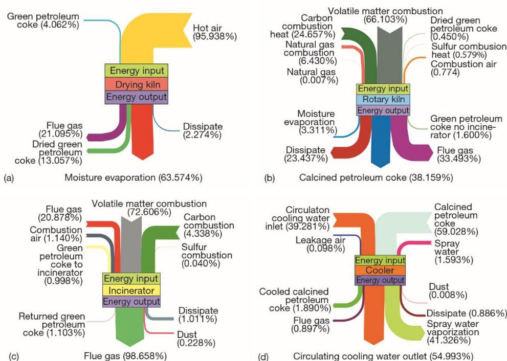
**Figure 3. Sankey diagram of energy flow in the four different equipment; (a) Sankey diagram of the energy flow in the drying kiln, (b) Sankey diagram of the energy flow in the rotary kiln, (c) Sankey diagram of the energy flow in the incinerator, and (d) Sankey diagram of the energy flow in the cooler**
