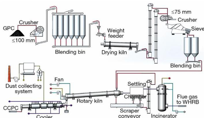
Figure 1. A schematic of the calcination process
