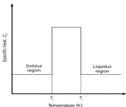
Figure 4. Graphical representation of the variation of specific heat with respect to temperature
