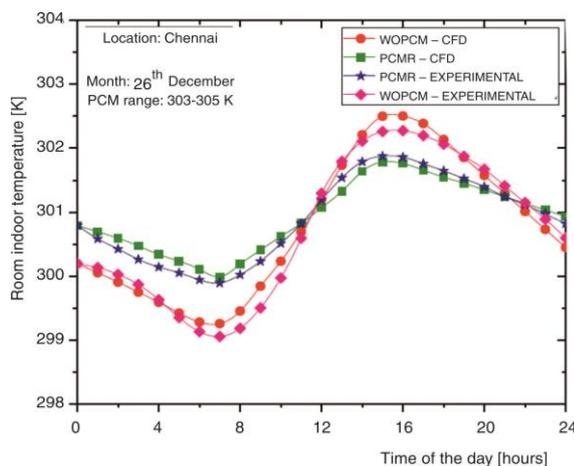
Figure 12. Validation of simulation results with experimental data
