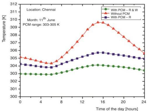
**Figure 9. Indoor temperature variation in building on 11<sup>th</sup> June**
