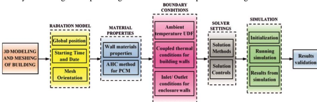
Figure 1. Scheme describing the methodology of simulation
