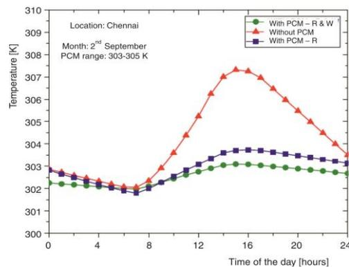
**Figure 8. Indoor temperature variation in building on 2<sup>nd</sup> September**
