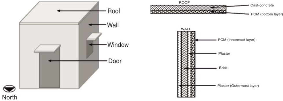
**Figure 3. Schematic view of the modelled building; (a) building model and (b) layers in walls and roof**
