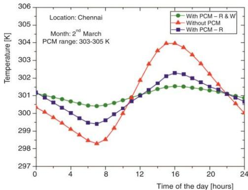
**Figure 7. Indoor temperature variation in building on 2<sup>nd</sup> March**
