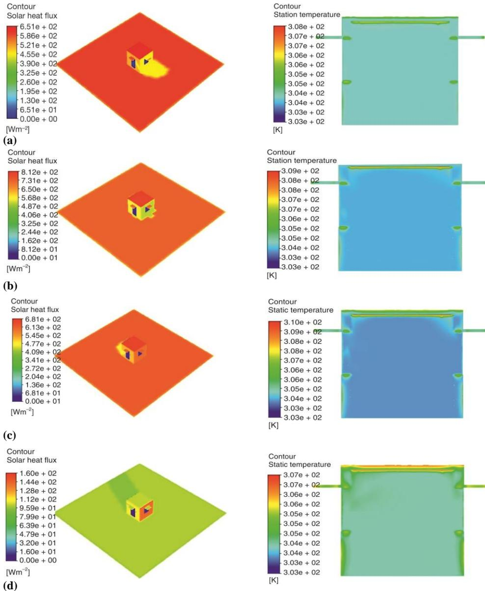
**Figure 6. Contours of solar heat flux incident on building walls and roof and cross sectional view of building indoor temperature; (a) Solar heat flux and cross-sectional view of indoor temperature at 9 a. m., (b) solar heat flux and cross-sectional view of indoor temperature at 12 noon, (c) solar heat flux and cross-sectional view of indoor temperature at 3 p. m., and (d) solar heat flux and cross-sectional view of indoor temperature at 6 p. m.**
