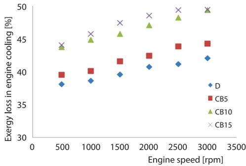
**Figure 6.** Influence of engine speed on exergy loss in engine cooling for the fuel samples
