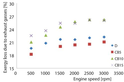
**Figure 7.** Influence of engine speed on exergy loss in exhaust gases for the fuel samples
