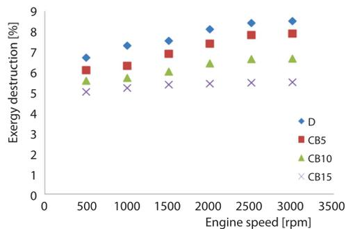
**Figure 8.** Influence of engine speed on exergy destruction the atmosphere for the fuel samples
