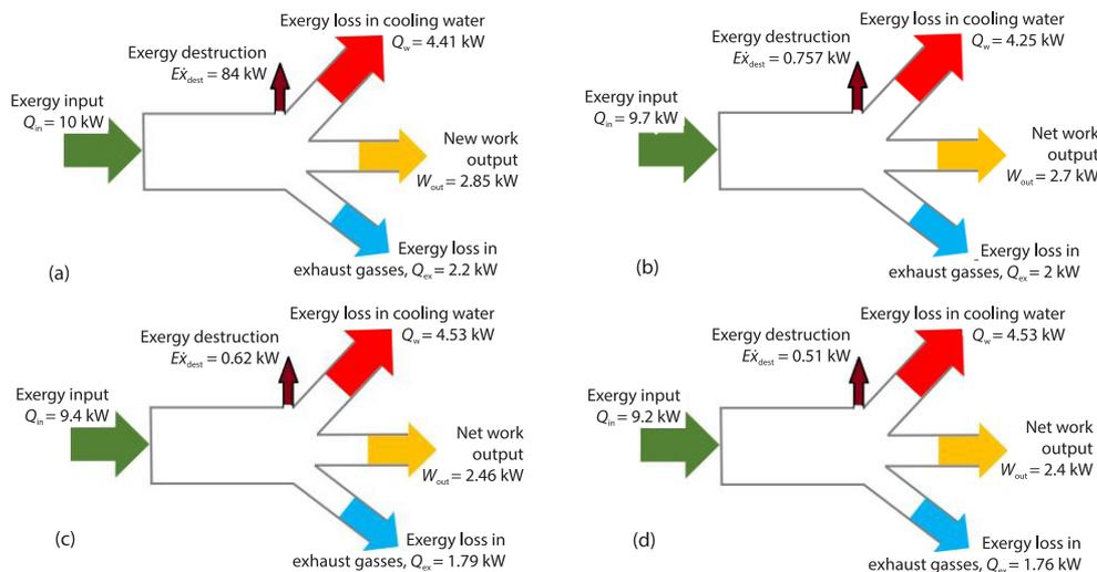
Figure 5. Exergy balance of DI diesel engine at 2500 rpm based on Second law of thermodynamics
