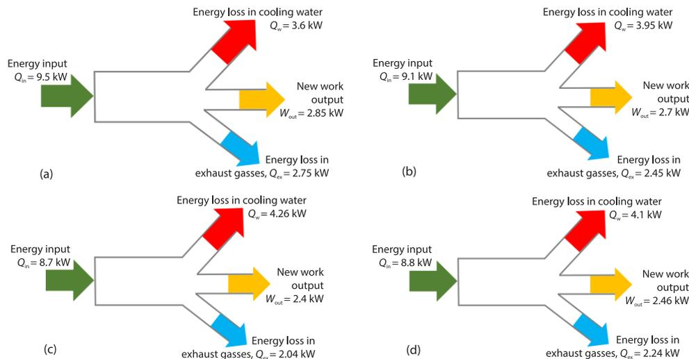
**Figure 3. Energy balance of DI diesel engine at 2500 rpm based on First law of thermodynamics; (a) D, (b) CB5, (c) CB10, and (d) CB15**
