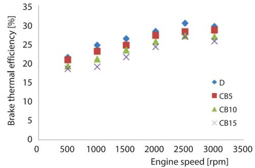
Figure 4. Influence of engine speed on brake thermal efficiency for the fuel samples
