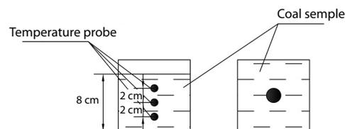
**Figure 2. Temperature measurement points**
