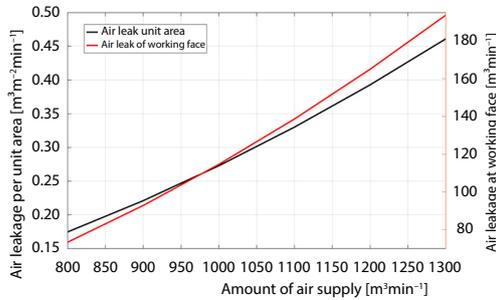
**Figure 7. Relationship between air leakage and air supply**
