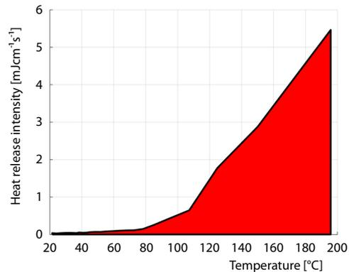
Figure 6. Variation of exothermic intensity of experimental coal sample
