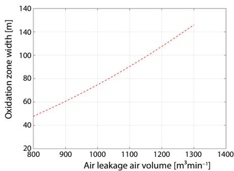
**Figure 8. Relationship between air supply and oxidation zone width**
