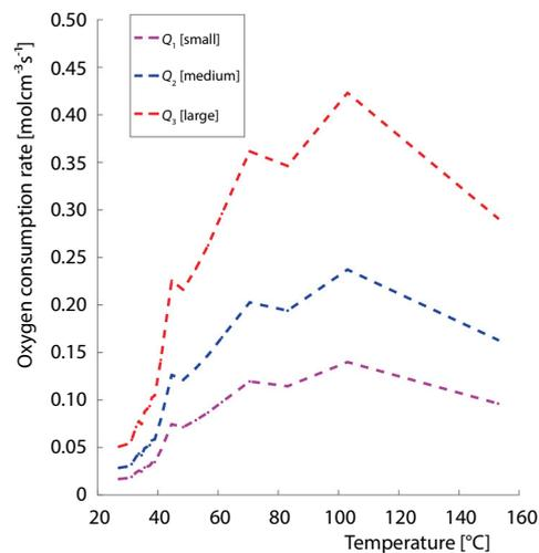
**Figure 4. Change in oxygen consumption rate for different air-leakage rates**
