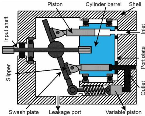
Figure 3. Schematic diagram of aircraft axial piston pump
