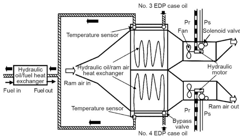
**Figure 5. Thermal management system in a hydraulic system of A380 civil aircraft**
