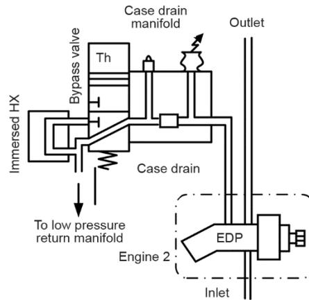
**Figure 4. Thermal management of A350 AHS; EDP – electric driven pump**
