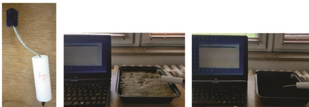
Figure 2. (a) Smart capacitive moisture sensor, (b) moisture measurement in the mineral wool sample, and (c) moisture measurement in the soil sample
