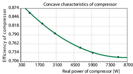
Figure 2. Concave efficiency-real power characteristics of the compressor
