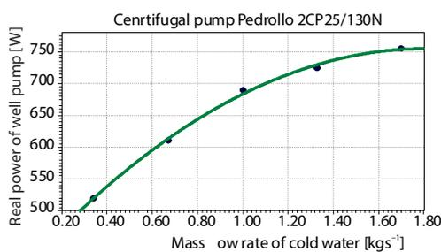
Figure 4. The efficiency-mass-flow rate characteristics of well pump
