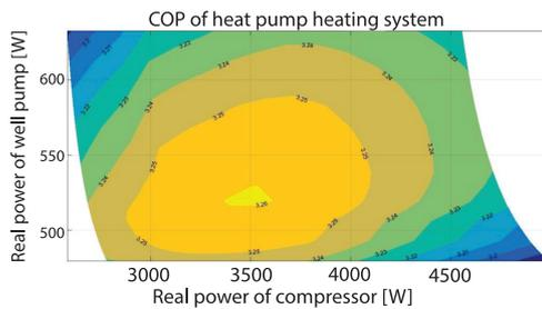
Figure 8. Isohyse of the COP depend on the compressor and well pump real power
