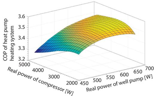
Figure 6. The COP and COP<sub>max</sub> of the cold water loop of the heat pump heating system with the convex efficiency characteristics of compressor
