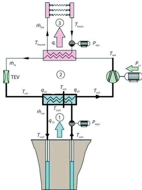
Figure 1. Physical system; 1 – cold water loop, 2 – refrigeration circuit, and 3 – warm water loop
