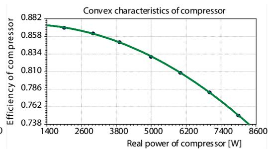
Figure 3. Convex efficiency-real power characteristics of the compressor
