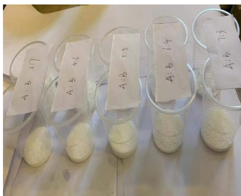
Fig. 1 Mixed samples of capric acid and palmitic acid with different mix proportion
