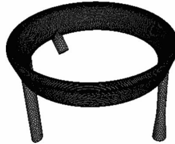
Figure 3. Piston cooling cavity mesh model
