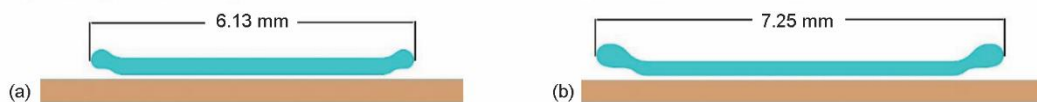
Figure 7. Sketch of the spreading of water and ethanol droplets; measurement of the spreading of ethanol and water droplets in the Leidenfrost state at the same surface aluminum temperature 270 °C; both droplets have the same initial diameter 2.7 mm and the impacting velocity is low 0.27 m/s; ethanol droplet spreads more than water droplet; the sketch is not to scale: (a) spreading of water droplet and (b) spreading of ethanol droplet
