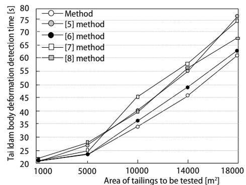
**Figure 8. Comparison of deformation speed detection of tailings dam**
