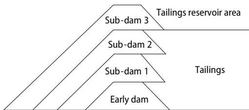
**Figure 1. Dam construction method of midline tailings**
