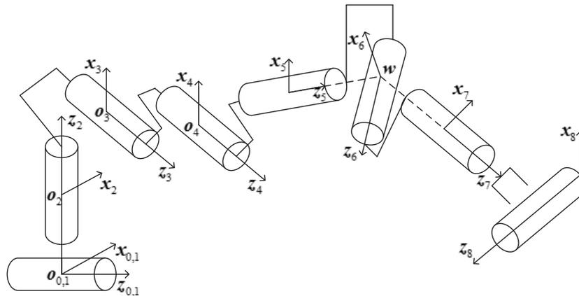
Figure 2. Plasma redundant robot co-ordinate system
