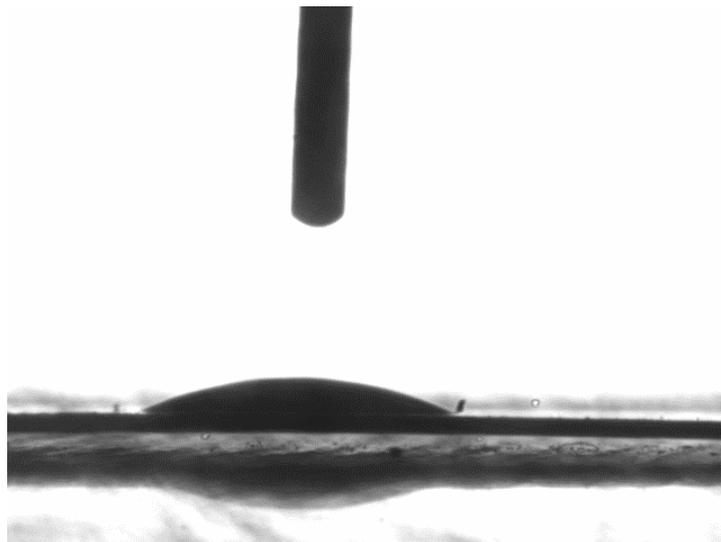
**Figure 5. Diagram of water drop angle optimization test**
