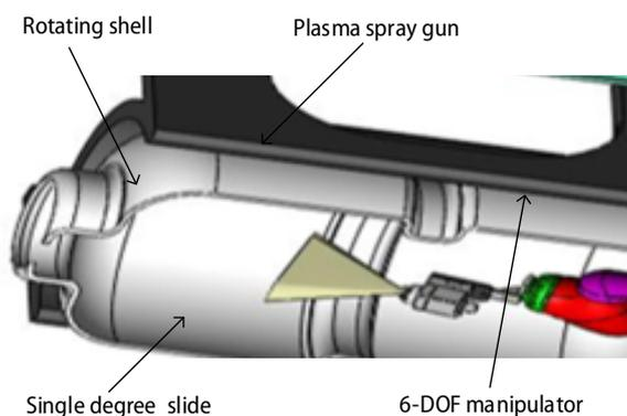
Figure 1. Model of plasma redundant robot
