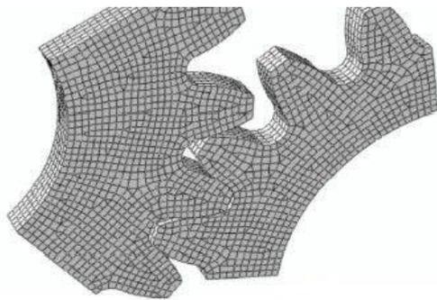
**Figure 1. Finite element model for gear pair meshing**
