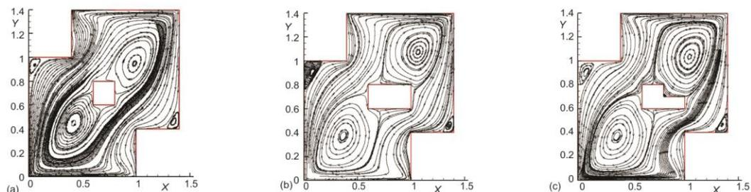
**Figure 4(C).** Comparison of streamlines for a double lid driven cavity with both parallel and anti-parallel wall motion; horizontal and vertical velocities along mid width:  $Re = 400$ , (a)  $AR = H/L = 0.5$ , (b)  $H/L = 1$ , and (c)  $H/L = 2$
