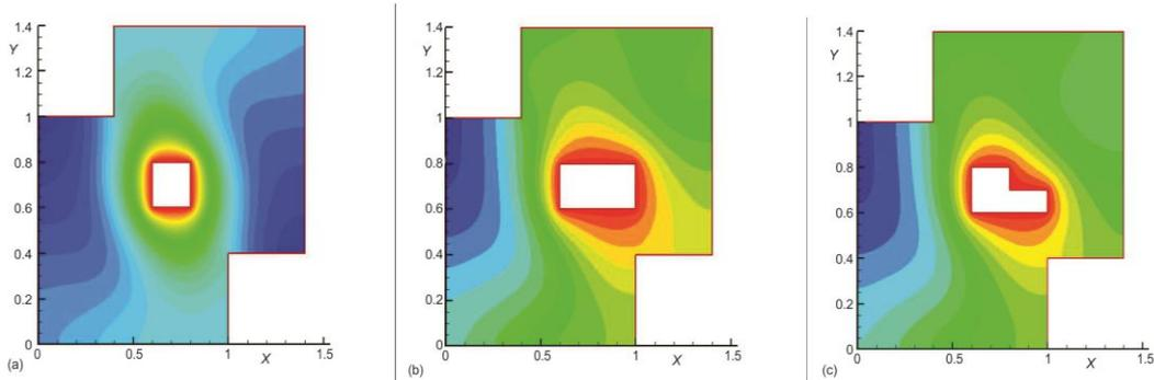
**Figure 3. Temperature contour of double lid driven staggered cavity both parallel and anti-parallel wall motion; horizontal and vertical velocity along mid width:  $Re = 50$ , (a)  $H/L = 1$ , (b)  $H/L = 0.5$ , and (c)  $H/L = 2$**
