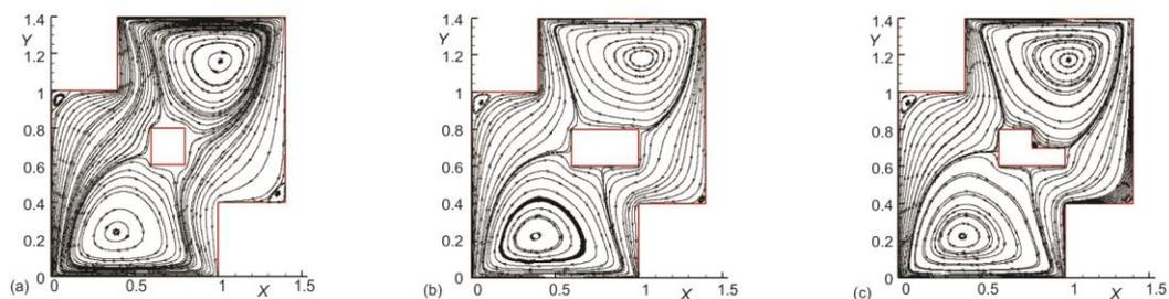
**Figure 4(B).** Comparison of streamlines for a double lid driven cavity with both parallel and anti-parallel wall motion; horizontal and vertical velocities along mid width:  $Re = 100$ , (a)  $AR = H/L = 0.5$ , (b)  $H/L = 1$ , and (c)  $H/L = 2$
