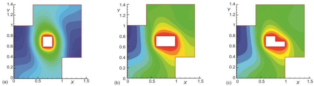
**Figure 5(A).** Comparison of temperature Contour for a double lid driven cavity with both parallel and anti-parallel wallmotion; horizontal and vertical velocities along mid width:  $Re = 50$ , (a)  $AR = H/L = 0.5$ , (b)  $H/L = 1$ , and (c)  $H/L = 2$
