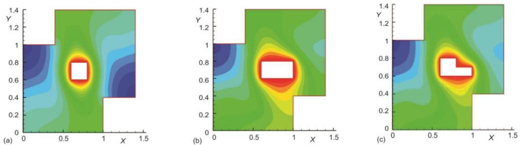
**Figure 5(B).** Comparison of temperature Contour for a double lid driven cavity with both parallel and anti-parallel wallmotion; horizontal and vertical velocities along mid width:  $Re = 100$ , (a)  $AR = H/L = 0.5$ , (b)  $H/L = 1$ , and (c)  $H/L = 2$
