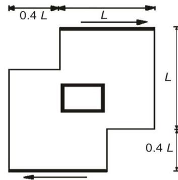
**Figure 1. Schematic diagram of block located two sided lid driven staggered cavity with parallel and anti-parallel wall motion**
