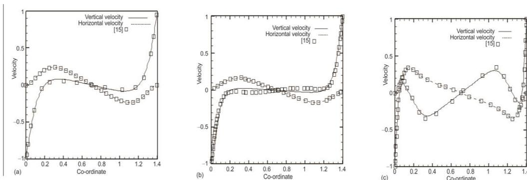
**Figure 2. Comparison of velocities for a double lid driven cavity both parallel and anti-parallel wall motion; horizontal and vertical velocity along mid width: (a)  $Re = 50$ , (b)  $Re = 100$ , and (c)  $Re = 1000$**
