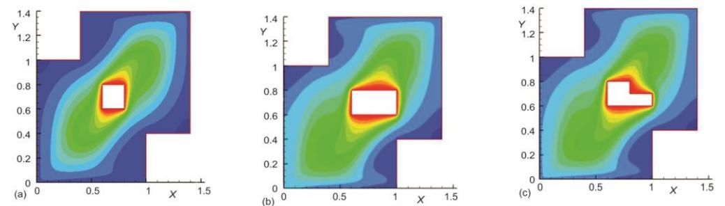
**Figure 5(D).** Comparison of temperature Contour for a double lid driven cavity with both parallel and anti-parallel wallmotion; horizontal and vertical velocities along mid width:  $Re = 1000$ , (a)  $AR = H/L = 0.5$ , (b)  $H/L = 1$ , and (c)  $H/L = 2$
