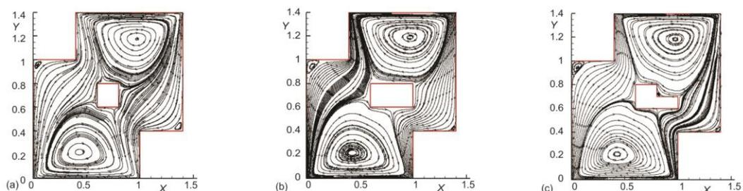
**Figure 4(A).** Comparison of streamlines for a double lid driven cavity with both parallel and anti-parallel wall motion; horizontal and vertical velocities along mid width:  $Re = 50$ , (a)  $AR = H/L = 0.5$ , (b)  $H/L = 1$ , and (c)  $H/L = 2$
