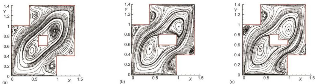
**Figure 4(D).** Comparison of streamlines for a double lid driven cavity with both parallel and anti-parallel wall motion; horizontal and vertical velocities along mid width:  $Re = 1000$ , (a)  $AR = H/L = 0.5$ , (b)  $H/L = 1$ , and (c)  $H/L = 2$
