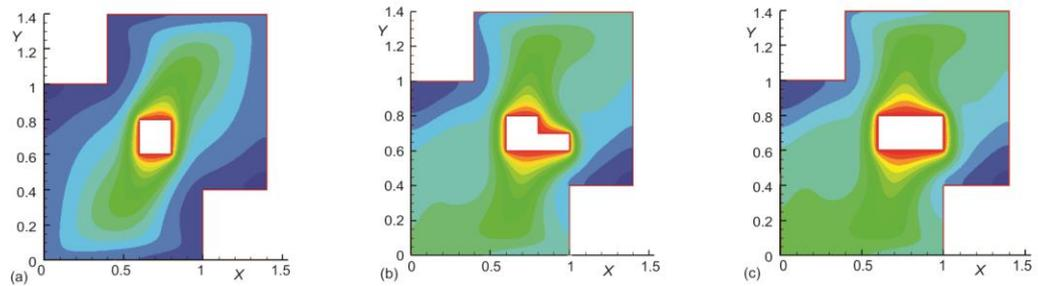
**Figure 5(C).** Comparison of temperature Contour for a double lid driven cavity with both parallel and anti-parallel wallmotion; horizontal and vertical velocities along mid width:  $Re = 400$ , (a)  $AR = H/L = 0.5$ , (b)  $H/L = 1$ , and (c)  $H/L = 2$
