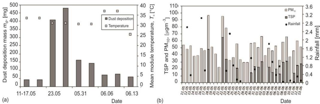
Figure 2. Dust deposited mass and the PV module temperature (a) and TSP, PM10, rainfall (b)
