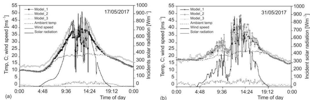
Figure 5. The PV module temperature for two days, calculated using three different models
