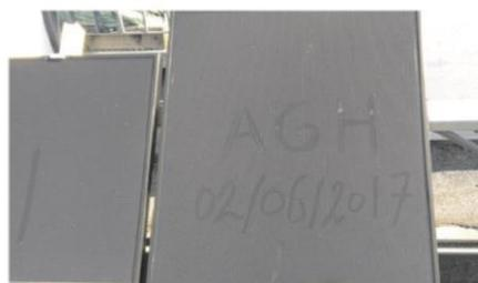
**Figure 1. An example of dust deposition on the module surface**
