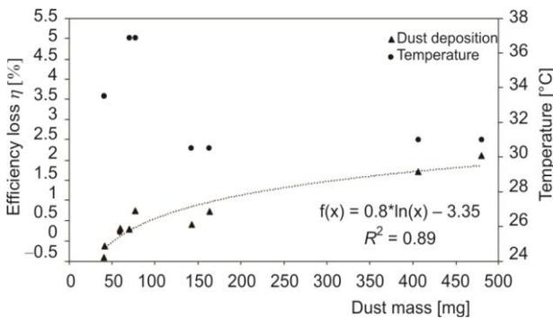
Figure 8. The average energy loss due to the natural dust deposition and module temperature
