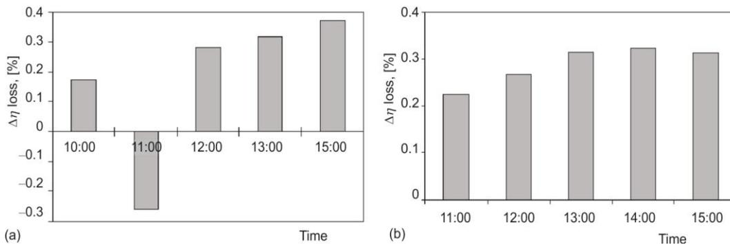
Figure 7. The PV system efficiency loss for cloudy (a) and sunny (b) days
