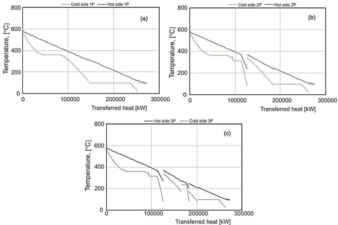
Figure 5. The  $q, T$  diagram for 1P (a), 2P (b), and 3P (c) heat recovery steam generator
