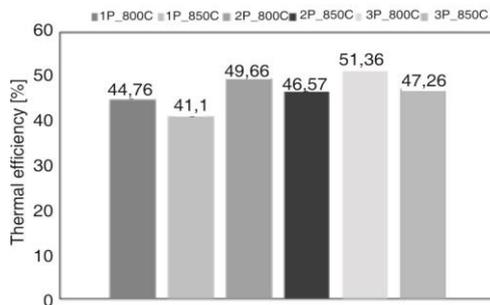
Figure 7. The thermal efficiency comparison between 1P, 2P, and 3P systems for cases 800 °C, 850 °C
