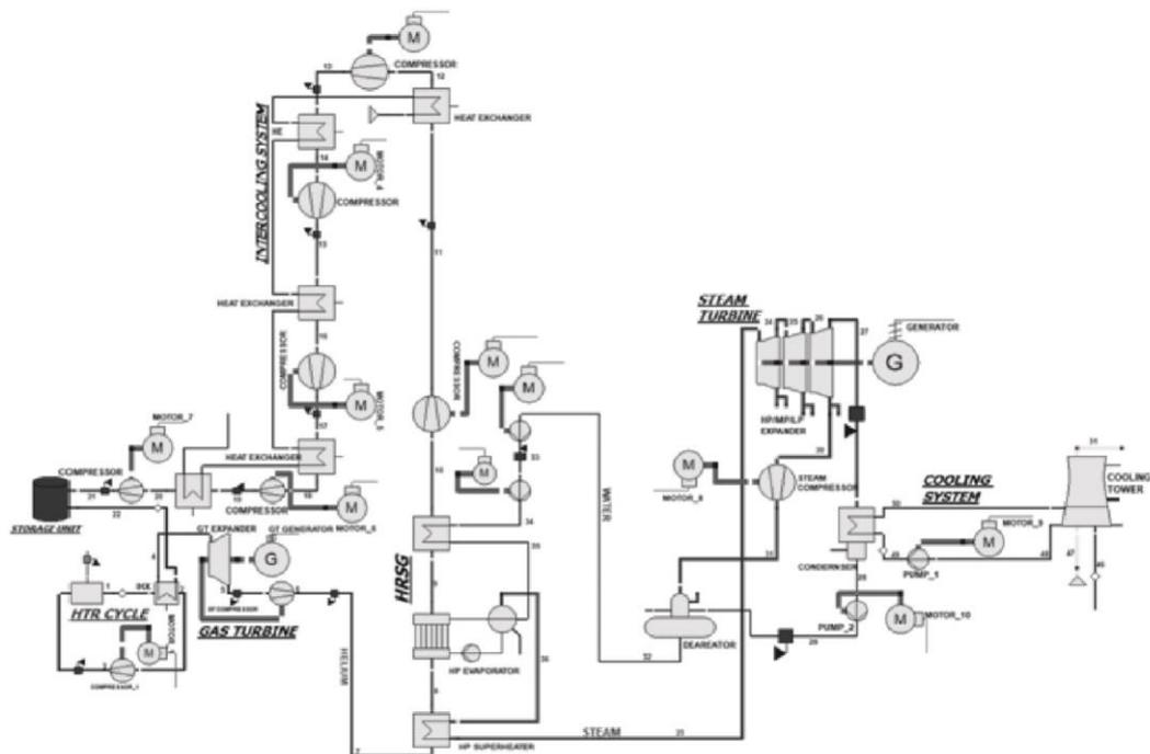
**Figure 1. Advanced GT combined cycle coupled with high temperature nuclear reactor and one pressure level heat recovery steam generator (1P HRSG)**
