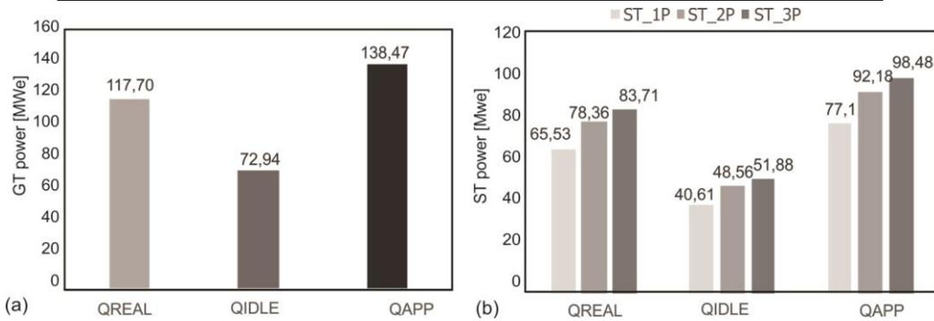
**Figure 3. The power of a GT (a) and steam turbine (b) divided into real, idle, and apparent electrical part**
