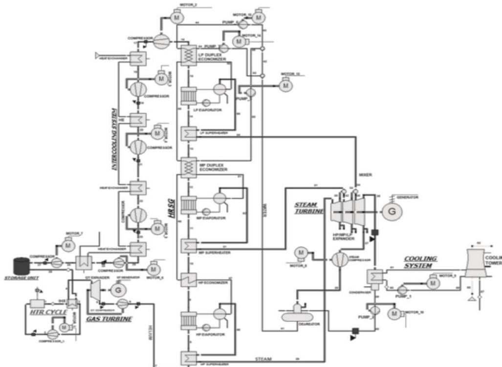
Figure 2. Advanced GT combined cycle coupled with high temperature nuclear reactor and three pressure level heat recovery steam generator (3P HRSG)
