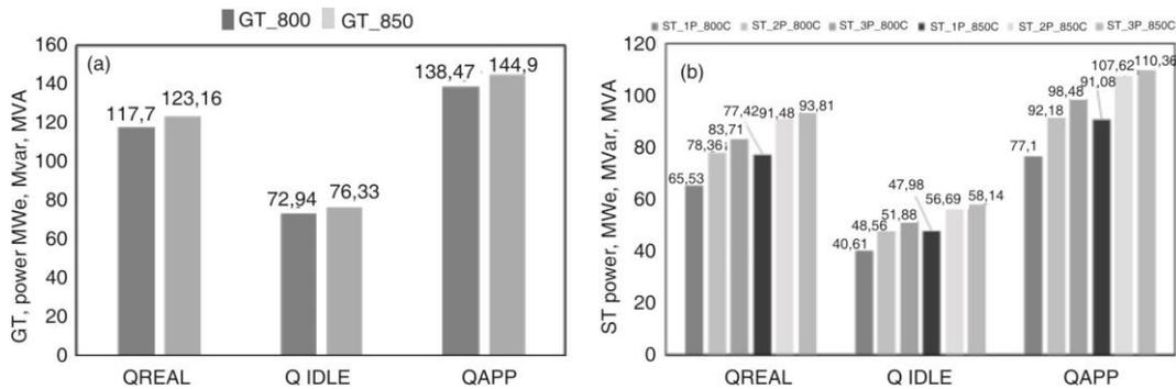
Figure 6. The real, idle, and apparent power of GT (a) and steam turbine for cases 800 °C, 850 °C
