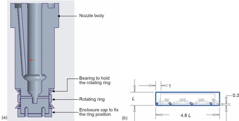
Figure 1. (a) Cut section, (b) nozzle ring
