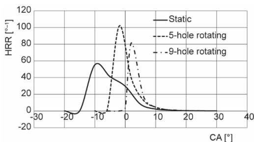
Figure 6. Heat release rate vs. CA
