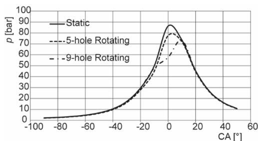
Figure 5. Cylinder pressure vs. CA
