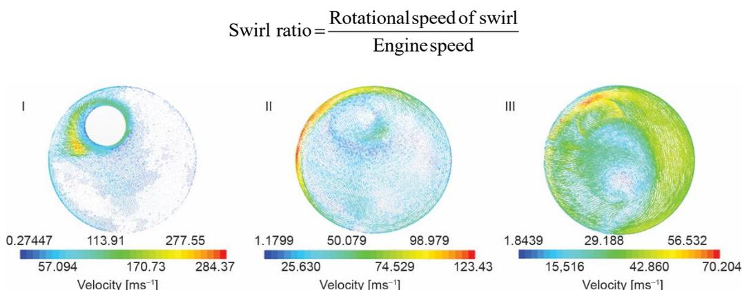
Figure 5. Velocity swirl disk at different length of stroke; SL – 11 mm, SL – 55 mm, SL – 110 mm
