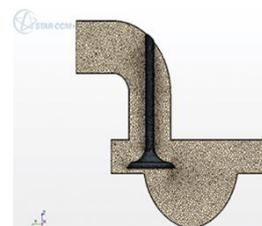
**Figure 3. Computational mesh of direct intake port**
