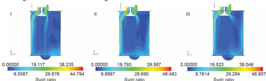
Figure 6. Swirl ratio of helical ports; Case I:  $\beta = 120^\circ$ , Case II:  $\beta = 150^\circ$ , Case III:  $\beta = 180^\circ$
