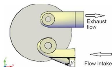
**Figure 1. Top view of helical port geometry**
