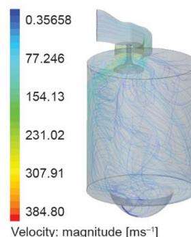
**Figure 8. Streamline path of intake charge during suction stroke**
