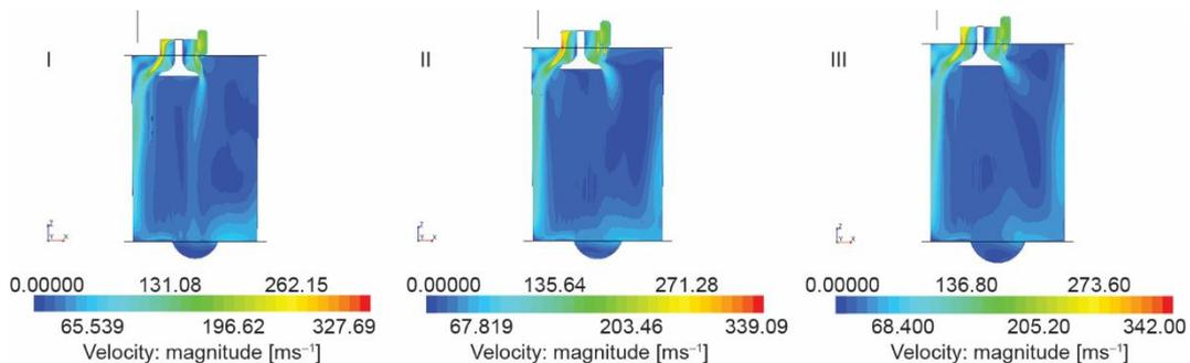
**Figure 4.** Velocity profiles of helical ports; Case I:  $\beta = 120^\circ$ , Case II:  $\beta = 150^\circ$ , Case III:  $\beta = 180^\circ$
