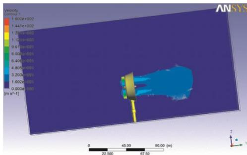
**Figure 1. Illustration of the fluid-flow within the blower housing** (for color image see journal web site)
