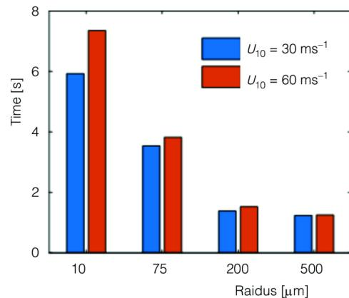
**Figure 5. Particle suspension time in different radii and different wind speeds**
