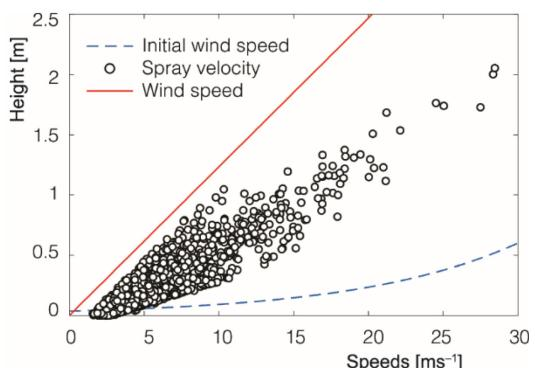
**Figure 6. Spray velocity and the profiles of wind speed in height direction**
