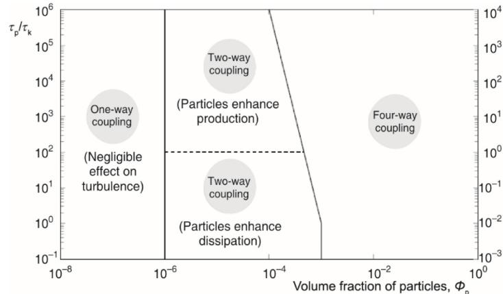
Figure 1. Classification of phase-coupling mechanisms
