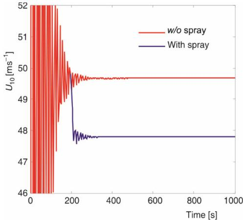
**Figure 2. Mean wind speed at  $z = 10$  m**
