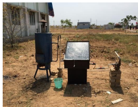
Figure 1. Photograph of the experimental set-up of stepped-cup solar still with biomass
