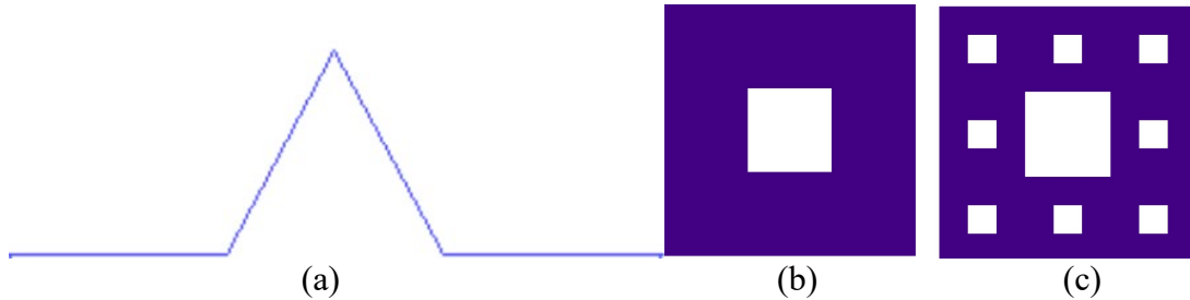
Fig. 2 First iteration of the Koch curve (a) and the Sierpinski carpet(b), Second iteration of the Sierpinski carpet(c).
