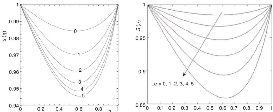
Figure 6. Density of motile microorganisms profile,  $S(\eta)$ , for different values of  $Le$  in the case of  $w = 1, Nt = Nb = 0.1, \beta = 1.5, Pe = Sc = Pr = 1$
