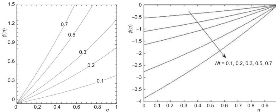
**Figure 3.** Nanoparticle volume fraction profile,  $\phi(\eta)$ , for different values of  $Nt$  in the case of  $w = 1$ ,  $Nb = 0.1$ ,  $\beta = 1.5$ ,  $Le = Pe = Sc = Pr = 1$
