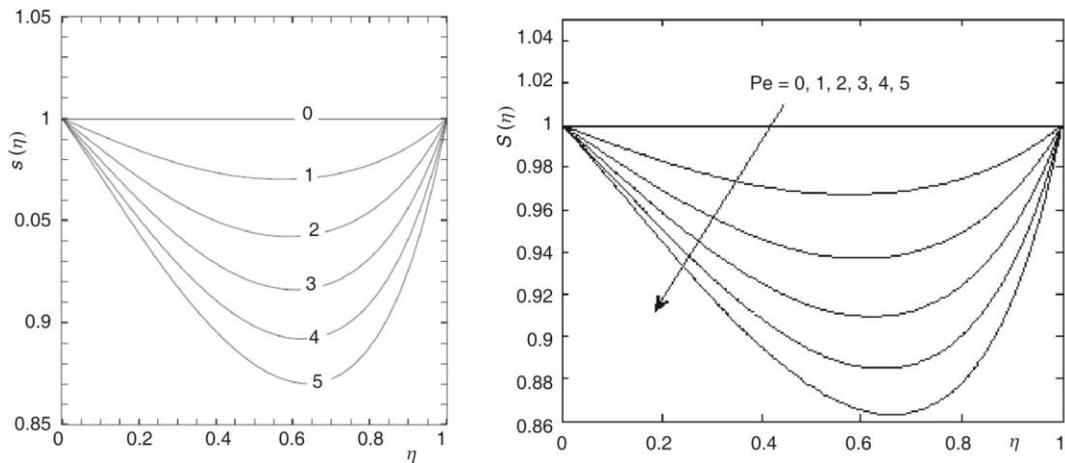
Figure 8. Density of motile microorganisms profile,  $S(\eta)$ , for different values of  $Pe$  in the case of  $w = 1$ ,  $Nt = Nb = 0.1$ ,  $\beta = 1.5$ ,  $Le = Pe = Sc = Pr = 1$
