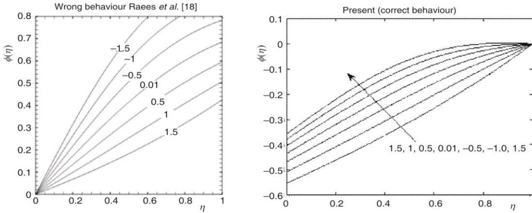
**Figure 1.** Nanoparticle volume fraction profile,  $\phi(\eta)$ , for different values of squeeze parameter,  $\beta$ , in the case of  $w = 1$ ,  $Nt = Nb = 0.1$ ,  $Le = Pe = Sc = Pr = 1$
