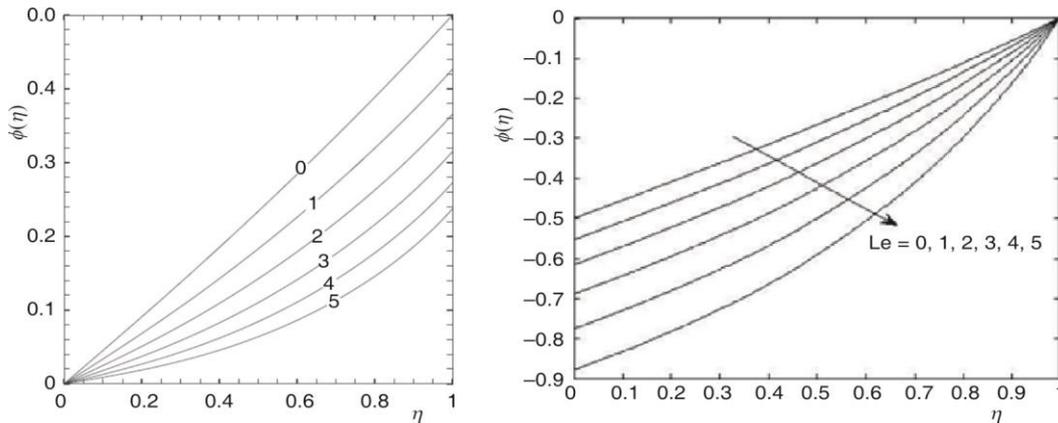
**Figure 2.** Nanoparticle volume fraction profile,  $\phi(\eta)$ , for different values of  $Le$  in the case of  $w = 1$ ,  $Nt = Nb = 0.1$ ,  $\beta = 1.5$ ,  $Pe = Sc = Pr = 1$
