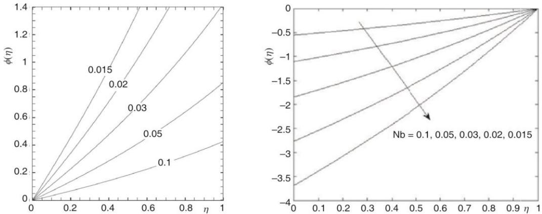
Figure 4. Nanoparticle volume fraction profile,  $\phi(\eta)$ , for different values of  $Nb$  in the case of  $w = 1, Nt = 0.1, \beta = 1.5, Le = Pe = Sc = Pr = 1$
