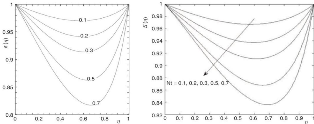
Figure 7. Density of motile microorganisms profile for,  $S(\eta)$ , different values of  $Nt$  in the case of  $w = 1$ ,  $Nb = 0.1$ ,  $\beta = 1.5$ ,  $Le = Pe = Sc = Pr = 1$
