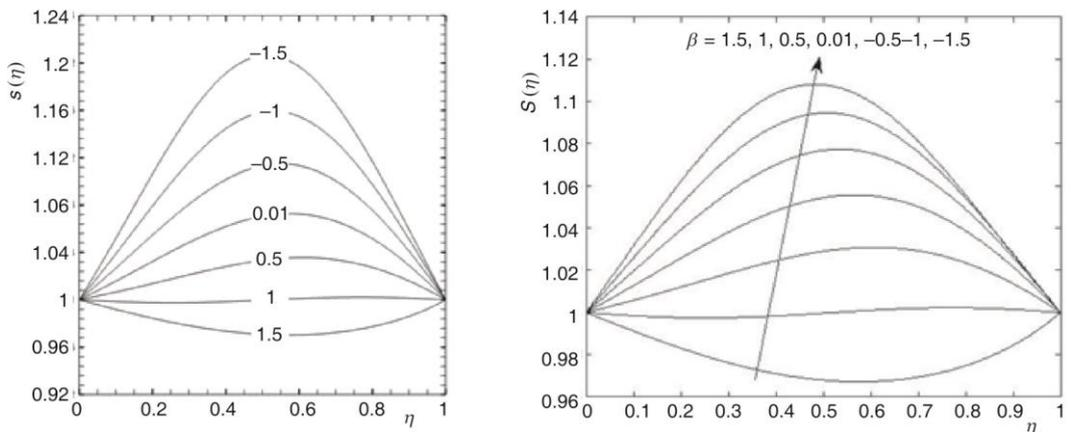
Figure 5. Density of motile microorganisms profile,  $S(\eta)$ , for different values of squeeze parameter,  $\beta$ , in the case of  $w = 1, Nt = Nb = 0.1, Le = Pe = Sc = Pr = 1$
