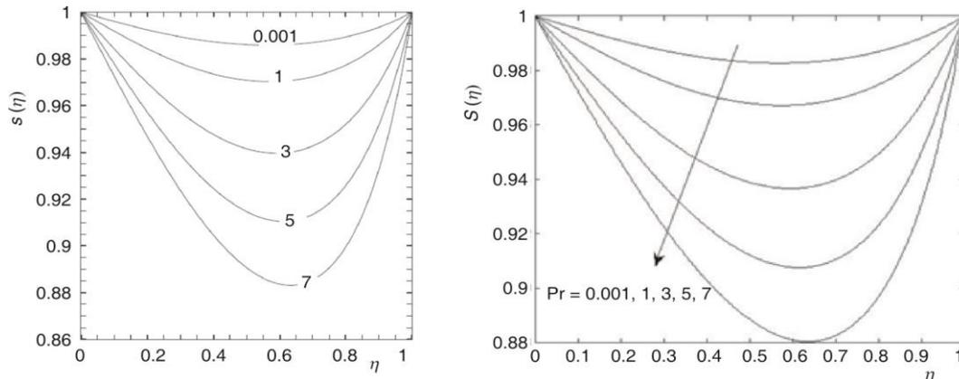
**Figure 10.** Density of motile microorganisms profile,  $S(\eta)$ , for different values of  $Pr$  in the case of  $w = 1$ ,  $Nb = Nt = 0.1$ ,  $\beta = 1.5$ ,  $Le = Pe = Sc = Pr = 1$
