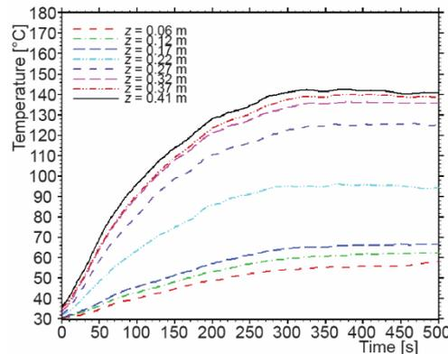
Figure 5. Profiles of temperature inside the experimental domain at different heights while using the fuel pan of diameter 0.097 m
