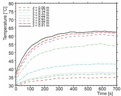
Figure 8. Profiles of temperature inside the experimental domain at different heights while using the fuel pan of diameter 0.053 m
