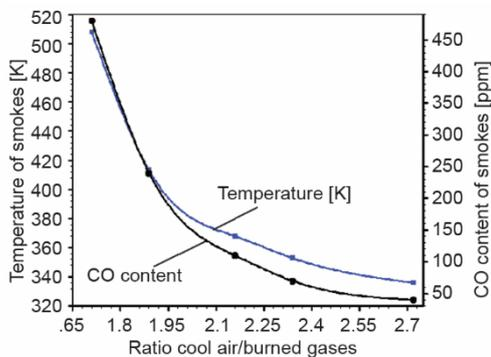
**Figure 10. Variation of CO content and temperature of smokes accumulated at the ceiling**
