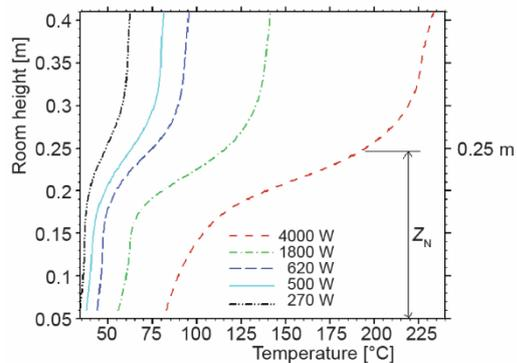
Figure 9. Vertical profiles of temperature during the steady-state at time  $t = 400$  seconds
