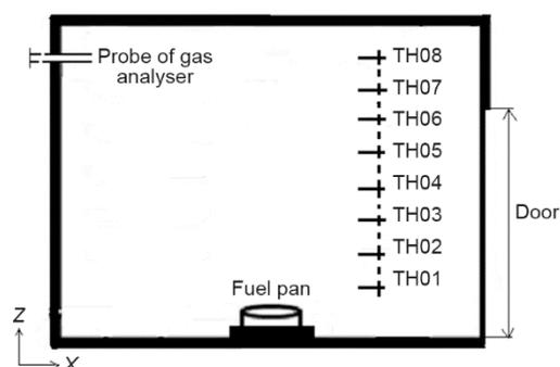
Figure 2. Locations of temperature sensors and fire source inside the domain
