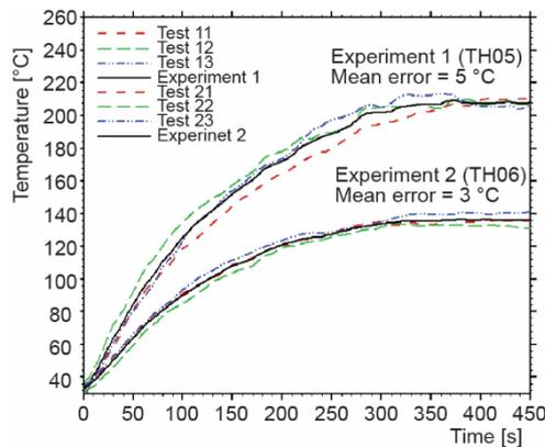
Figure 3. Illustration of the repeatability of experiments
