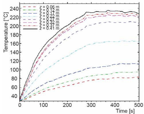
Figure 4. Profiles of temperature inside the experimental domain at different heights while using the fuel pan of diameter 0.130 m
