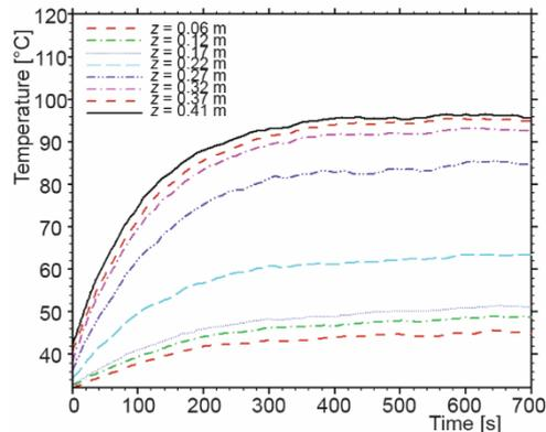
Figure 6. Profiles of temperature inside the experimental domain at different heights while using the fuel pan of diameter 0.075 m
