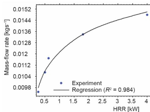
**Figure 11. Variation of the mass-flow rate of outgoing gases according to HRR**
