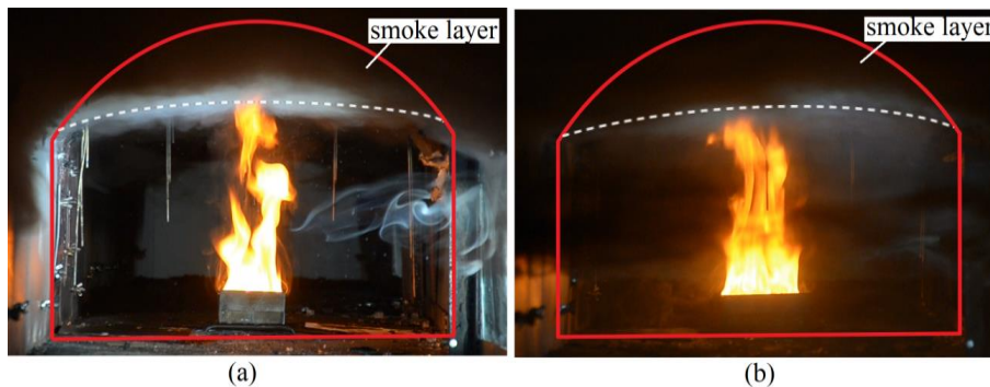
Fig. 8 Smoke layer and flame in diesel pool fires: (a) size A; (b) size B
