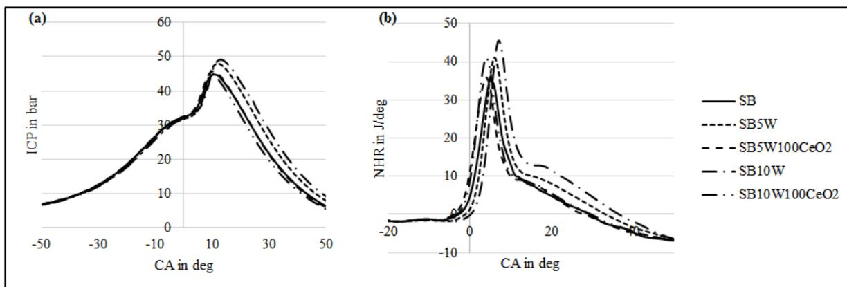
Fig.3. Combustion characteristics of test fuels: (a) ICP variation, and (b) NHR variation
