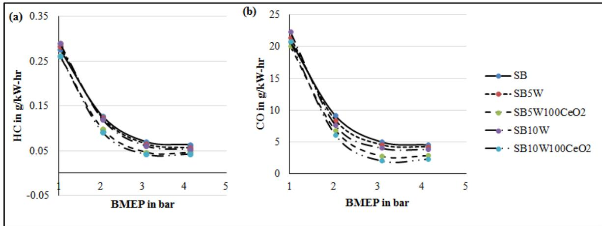
**Fig.6. Emission characteristics of test fuels: (a) HC, and (b) CO emission**
