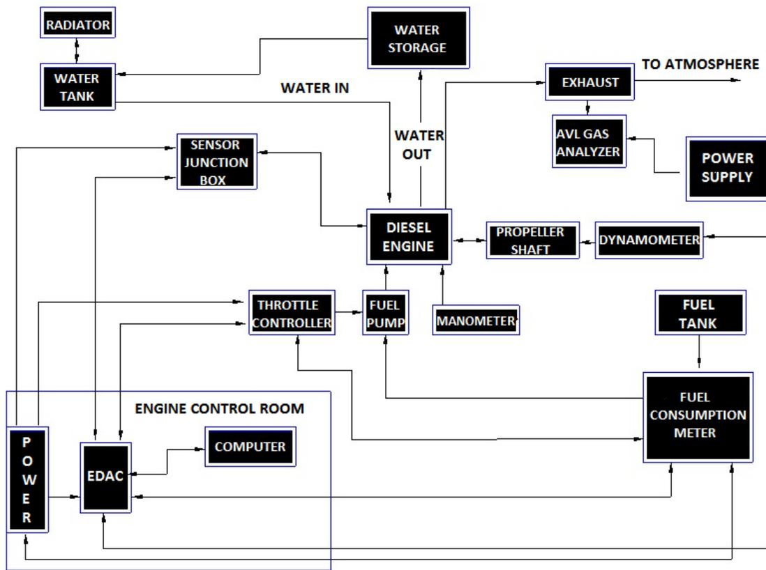
Fig.2. Schematic layout of the test engine setup
