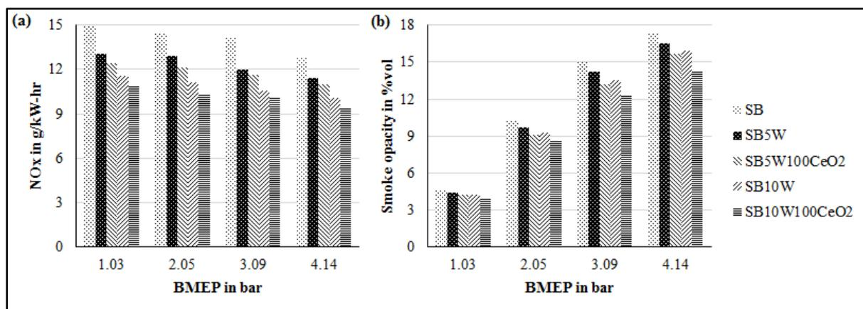
**Fig.5. Emission characteristics of test fuels: (a) NO<sub>x</sub>, and (b) Smoke emission**
