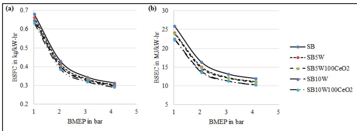
**Fig.4. Performance characteristics of test fuels: (a) BSFC, and (b) BSEC**
