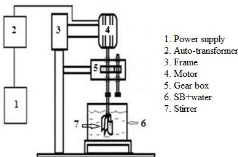
**Fig.1. Schematic layout of the emulsion preparation setup**
