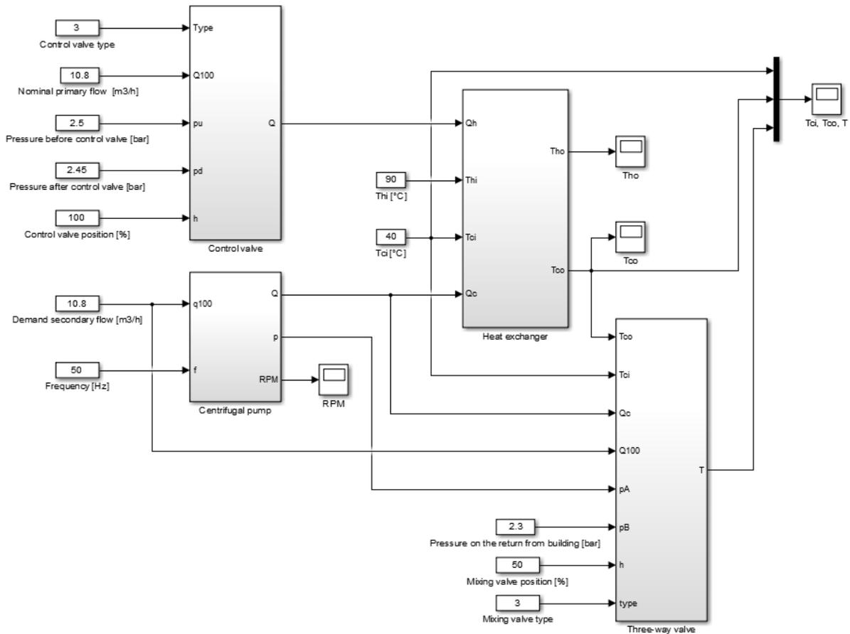
**Figure 3. Simulink® model of district heating substation**
