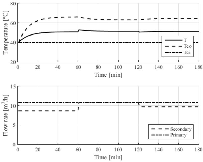
**Figure 7. Effect on the model output due to changes in the secondary flow**
