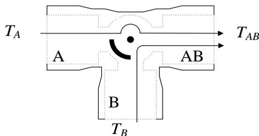
**Figure 2. Cross section of three-way valve**
