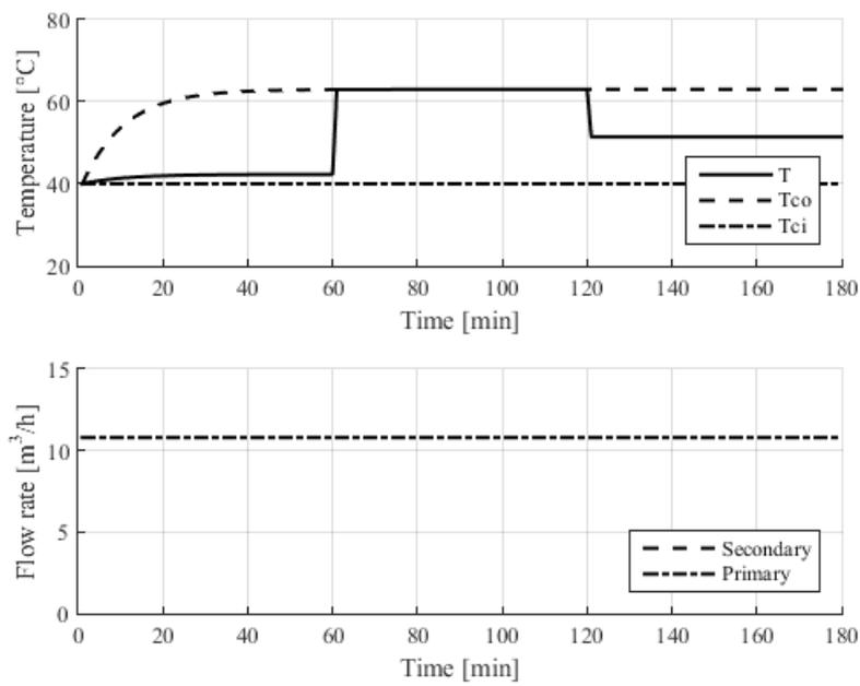
**Figure 8. Effect on the model output due to relative position of the three-way valve**
