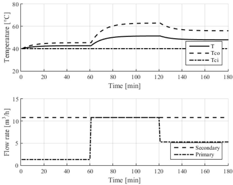
**Figure 6. Effect on the model output due to the changes in the primary flow**
