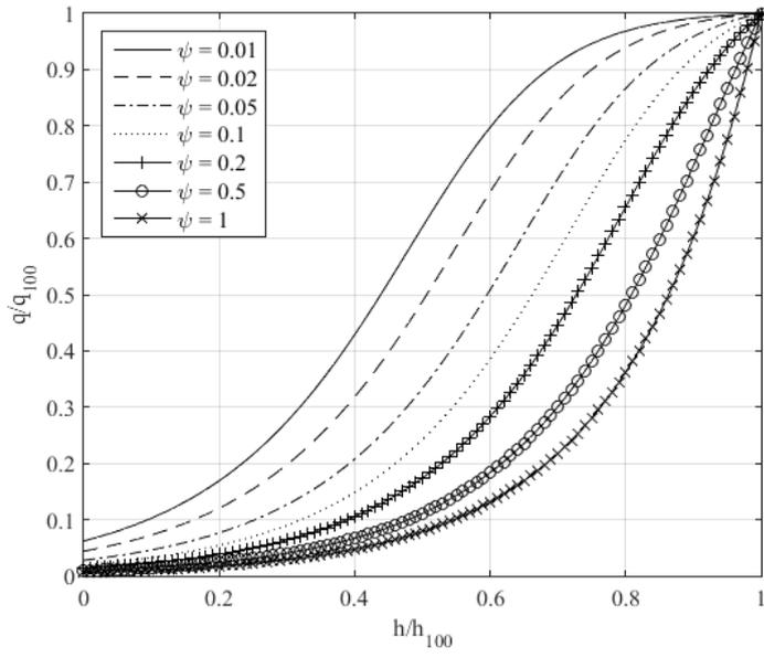
**Figure 4. Installed characteristic for equal-percentage valve**
