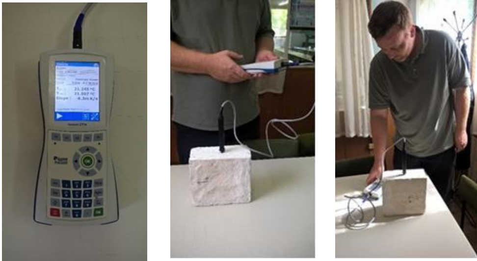
Figure 4 – The Isomet 2114 instrument for thermal conductivity measurements
