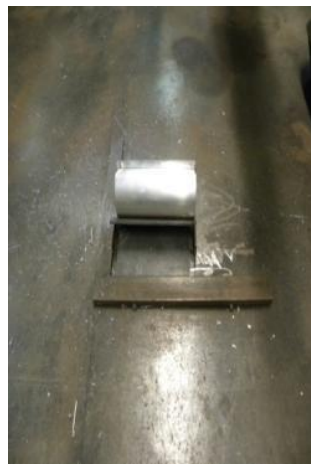
Fig. 2. Tube of 6063-T5 aluminium employed as base metal
