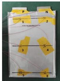
Fig.4 Lithium-ion batteries for laboratory use and their hot spot test lines
