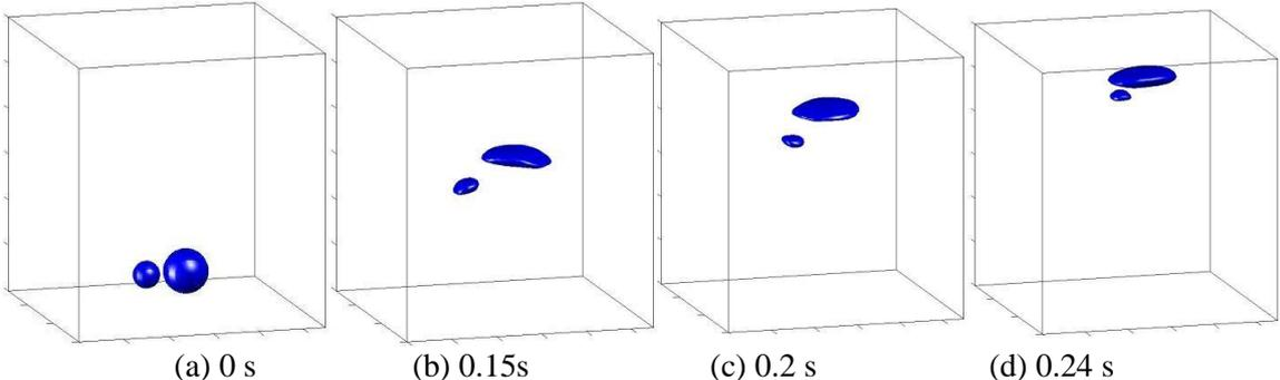
Fig. 7. The simulation of two horizontally arranged bubbles with incoordinate size
