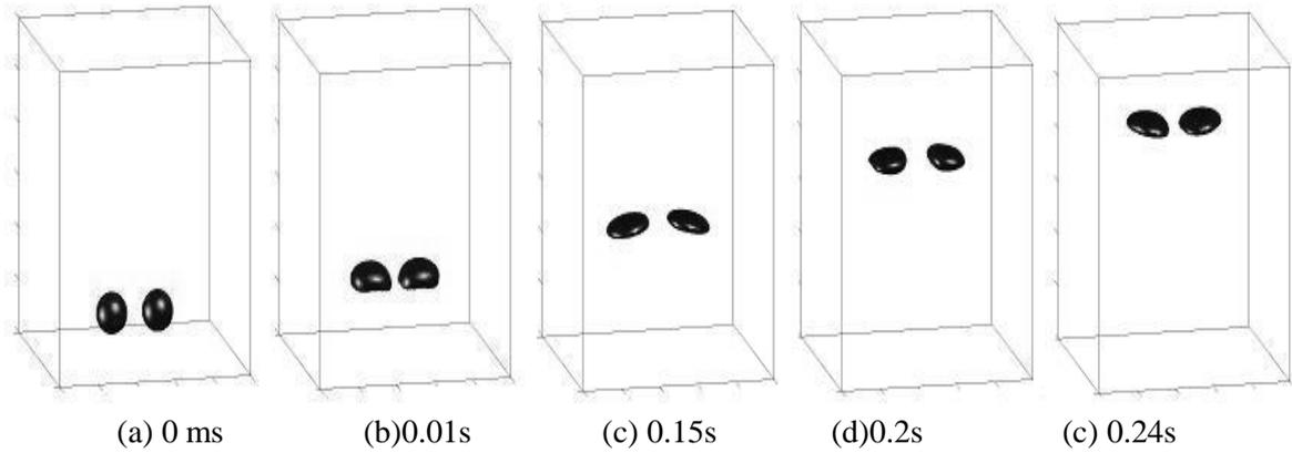
Fig. 4. Simulation of two bubble horizontally-arranged
