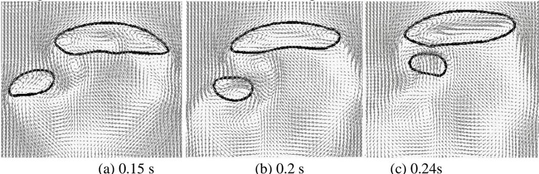
Fig. 8. The flow field of two bubbles in incoordinate size(distance=0.9cm)
