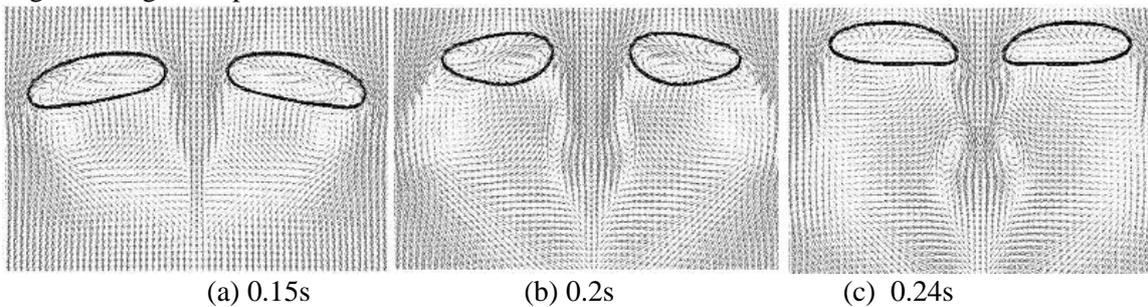
Fig. 6. The wake flow of the two bubbles
