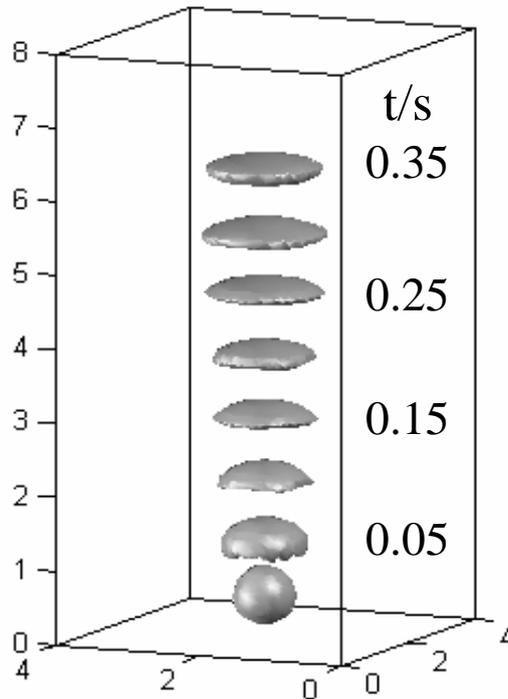
Fig. 1 The profile change of a rising bubble
