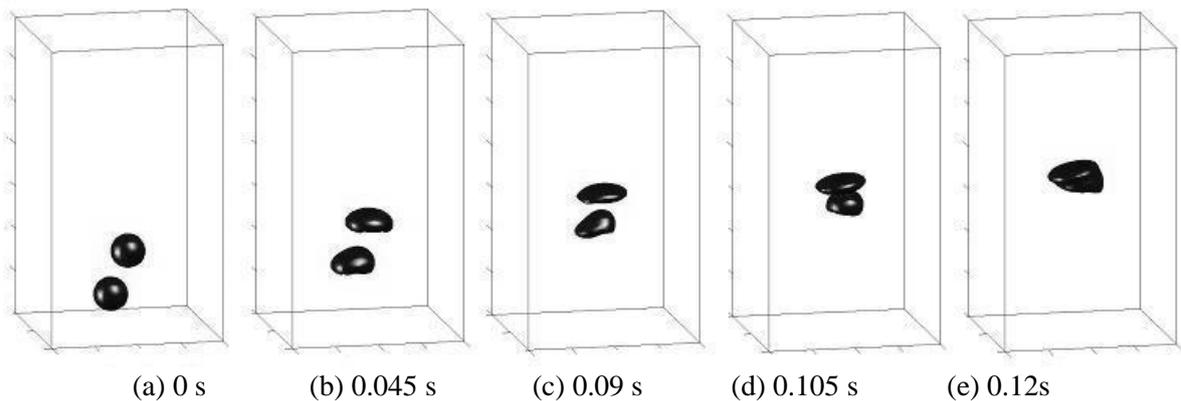
Fig. 11. The simulation of two vertically arranged bubbles
