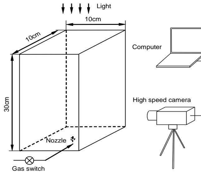
Fig. 3. Schematic diagram of high-speed camera experiment
