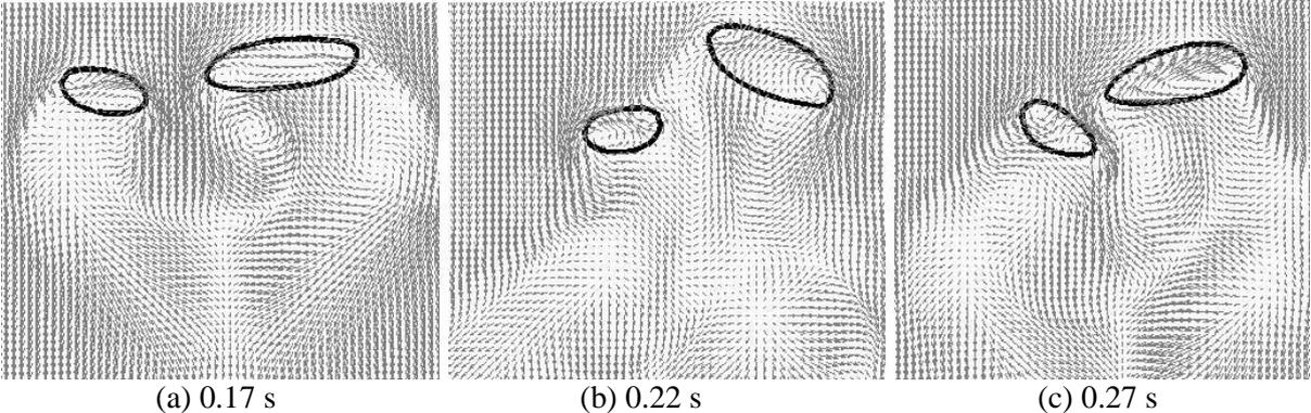
Fig. 9. The velocity field of two bubbles in incoordinate size (distance=1.2cm)
