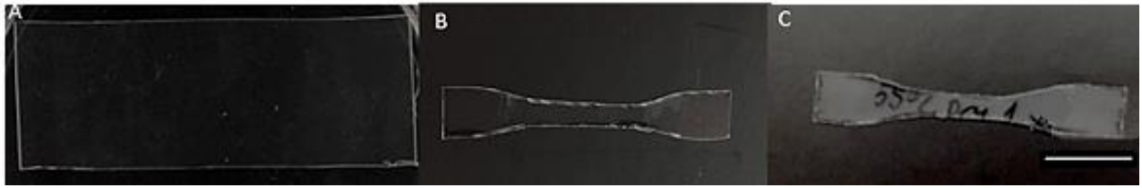
Figure 1. Physical changes in PLA films. (A) PLA1: initial films prior to mechanical tests (B) PLA2 dumb-bell: PLA films kept at room temperature for 5 years (C) PLA3 dumb-bell: PLA films pre-treated at 55°C for a year prior to 4 years of incubation at room temperature. Scale bar represents 1.5 cm.
