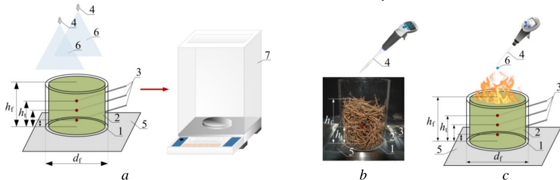
Fig. 1. Conventional scheme of experiments (without pyrolysis of FFM) under the influence of liquid aerosol (a) (1 – hollow cylinder with FFM sample; 2 – FFM; 3 – low-inertia thermocouples; 4 – spraying nozzle; 5 – grid (1×1 mm); 6 – aerosol, 7 – laboratory scales) and single drops (b, c) (model bed (b - sample in the initial state (not subjected to pyrolysis), c – FFM is thermally decomposing): 1 – hollow cylinder with FFM sample; 2 – FFM sample; 3 – low-inertia thermocouples; 4 – single-channel dispenser; 5 – grid (1×1 mm); 6 – drop of liquid)
