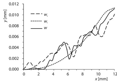
Figure 7. Comparison of theoretical and experimental values of opening displacement
