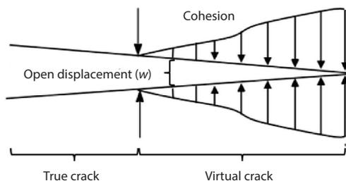
**Figure 1. Diagram of crack opening displacement**
