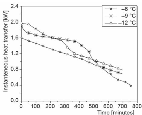
**Figure 6.** Instantaneous heat transfer in the storage tank for various bath temperatures (mass-flow rates of  $\dot{m} = 440\text{ Lph}$ )
