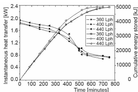
**Figure 8. Effect of mass-flow rate on instantaneous and cumulative heat transfer (HTF set point temperature  $-9\text{ }^{\circ}\text{C}$ )**
