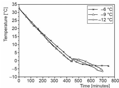
**Figure 5. Temperature time history of PCM at three different inlet HTF temperatures (mass-flow rate = 440 Lph)**
