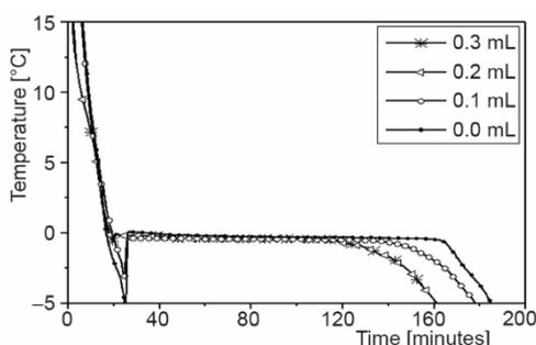
**Figure 4. Effect of pseudomonas concentration on temperature variation during freezing of PCM**
