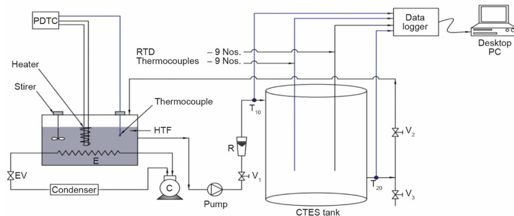
Figure 3. Schematic diagram of experimental set-up; E – evaporator, EV – expansion valve, C – compressor, R – rotameter,  $T_{10}$ - $T_{20}$  – thermocouples,  $V_1$ ,  $V_2$ ,  $V_3$  – valves
