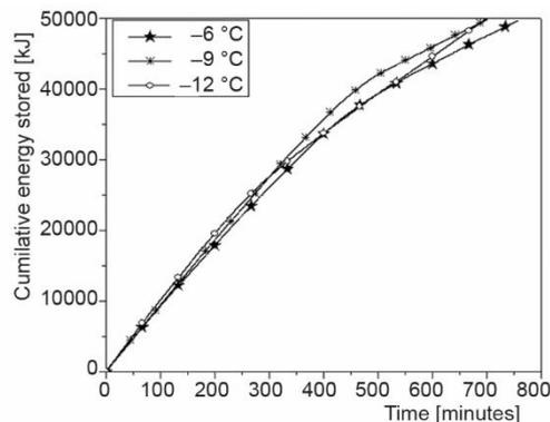
**Figure 7.** Cumulative energy stored in the storage tank for various bath temperatures (mass-flow rate  $\dot{m} = 440\text{ Lph}$ )
