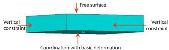
**Figure 4. Temperature stress calculation boundary conditions**
