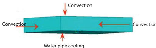
**Figure 3. Temperature calculation boundary conditions**
