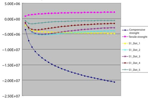
**Figure 11. Relationship between compressive tensile strength and the  $S_3$  of the first to 5<sup>th</sup> monitoring nodes**
