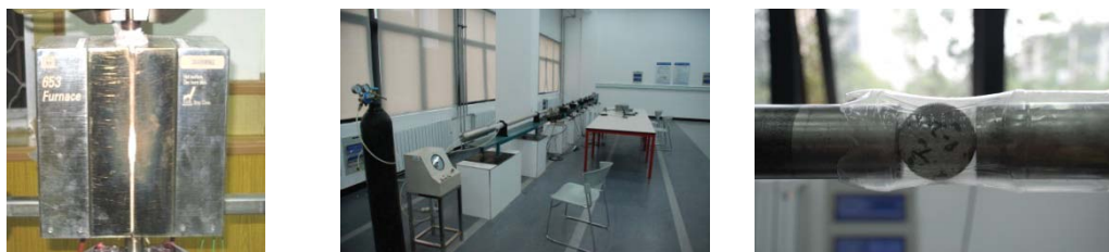
(a) MTS652.02 high temperature furnace (b) SHPB test system (c) Sample loading method
