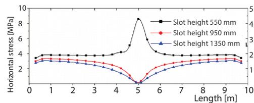
**Figure 10. Horizontal stress distribution of coal seam with different slot height (monitoring line  $H_3$ )**
