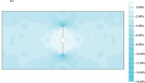
Figure 6. Contour of the horizontal stress
