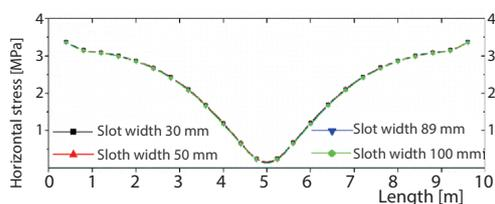
**Figure 9. Horizontal stress distribution of coal seam with different slot width (monitoring line  $H_3$ )**
