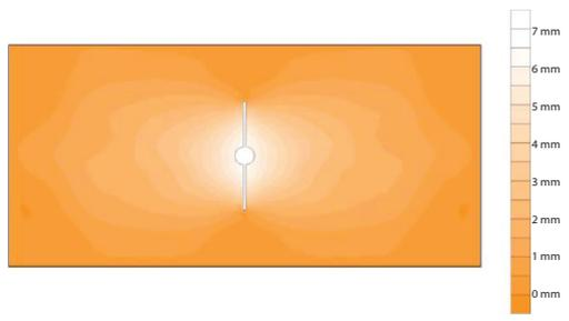
Figure 7. Contour of the horizontal displacement
