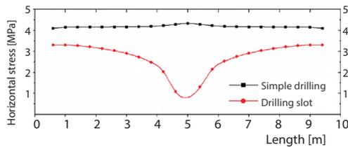
**Figure 8. Comparison of stress before and after slotted seam (monitoring line  $H_3$ )**
