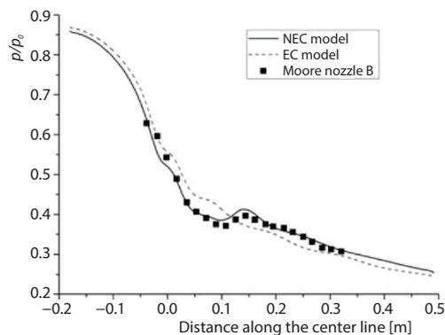
Figure 1. Comparison between the numerical and experimental results for distribution of pressure ratio along the centerline of the Moore's nozzle
