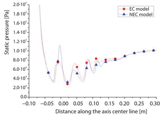
Figure 3. Static pressure distribution along the center line of two models
