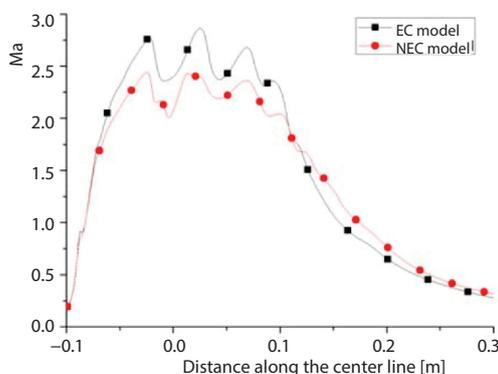
Figure 2. Mach number distribution along the center line of two models
