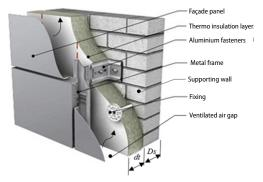
Figure 1. The principal scheme of the ventilated facades with aluminum fixing element
