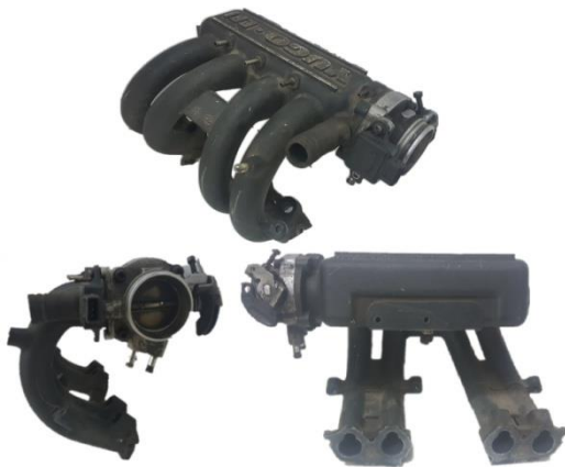
Figure 1. Intake manifold of the engine
