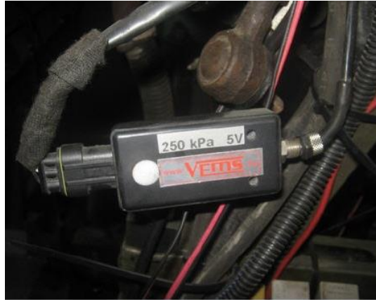
Figure 7. MAP sensor mounted on the engine [22]
