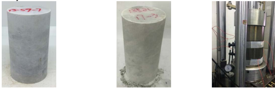
(a) Specimen for \sigma_3=6.3\text{MPa} (b) Specimen for \sigma_3=9.6\text{MPa} (c) Testing apparatus Figure 1. Specimens and apparatus for long-term triaxial creep experiments
