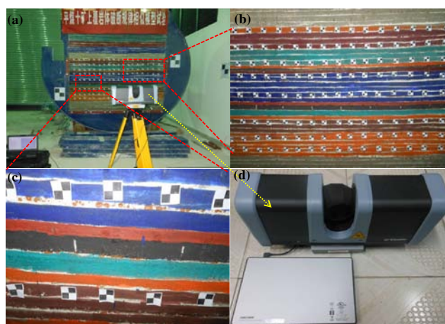
Fig. 3 Experimental model and system (a) Experimental system; (b) Displacement measuring point; (c) Quasi mining seam; (d) Trimble FX three-dimensional laser scanner
