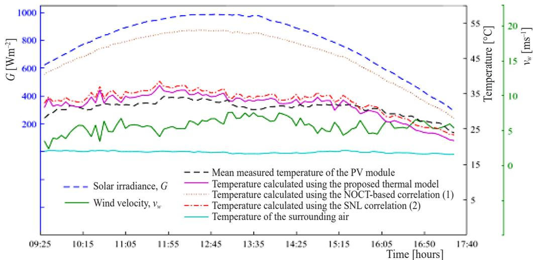
**Figure 5. Comparison between measured and calculated temperatures of the mono-crystalline PV module when it is inclined at an angle of 37° to the horizontal for different values of  $T_a$ ,  $v_w$ , and  $G$  [29]**
