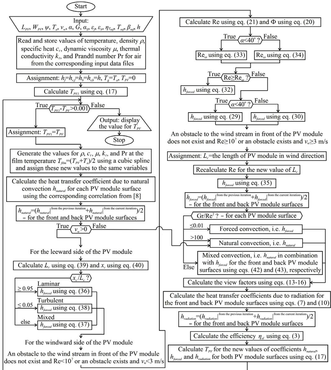
Figure 3. Flowchart of the proposed thermal model
