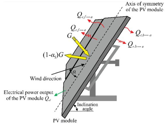
Figure 1. Illustration of the energy balance equation for the open-rack mounted PV module
