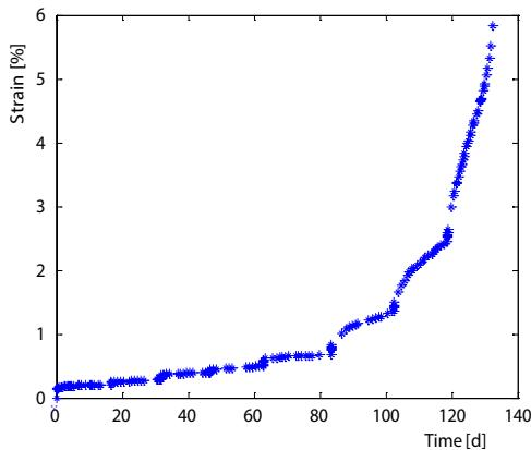
Figure 4. The whole-process creep curve
