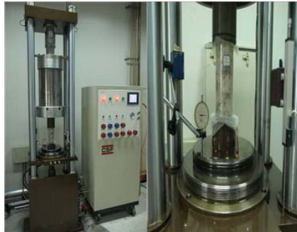
Fig. 3 Experimental setup of creep test of salt rock
