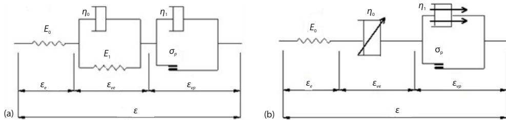
**Figure 2. Schematic view of the creep constitutive model; (a) Nishihara model, (b) fractional derivative model**
