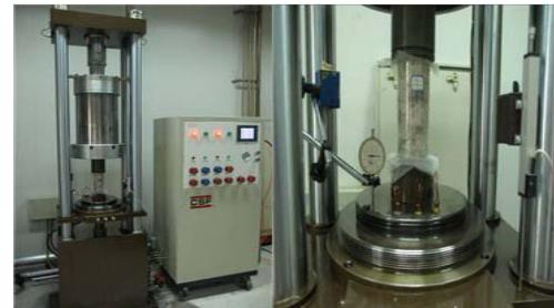
Figure 3. Experimental set-up of creep test of salt rock
