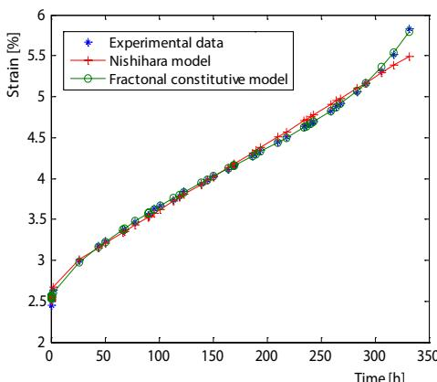
**Figure 5. Experimental data and the fitting curves obtained by the Nishihara model and the fractional derivative model**
