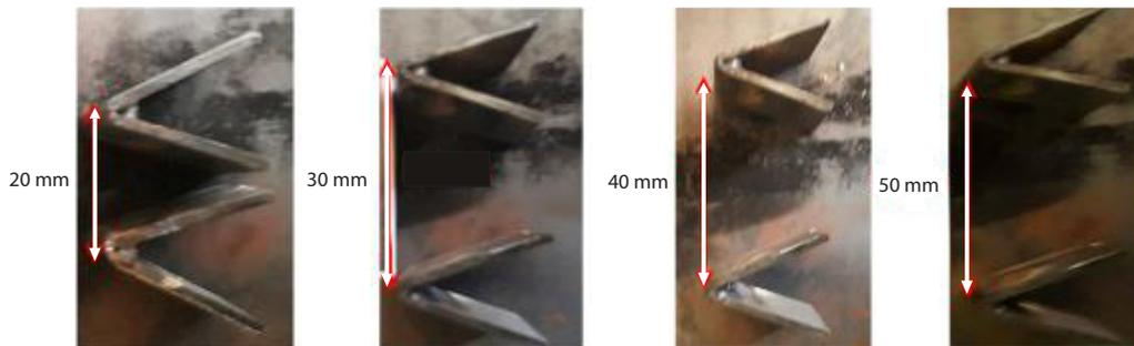
Figure 3. General view of V-gutter flame holders and the distances between them
