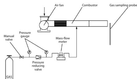
Figure 2. Schematic diagram of the experimental system (rear view)
