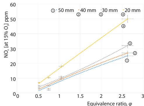
**Figure 5. Influence of the equivalence ratio on  $\text{NO}_x$  emissions**
